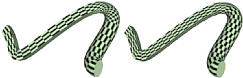
Before and after applying Normalize to loft
