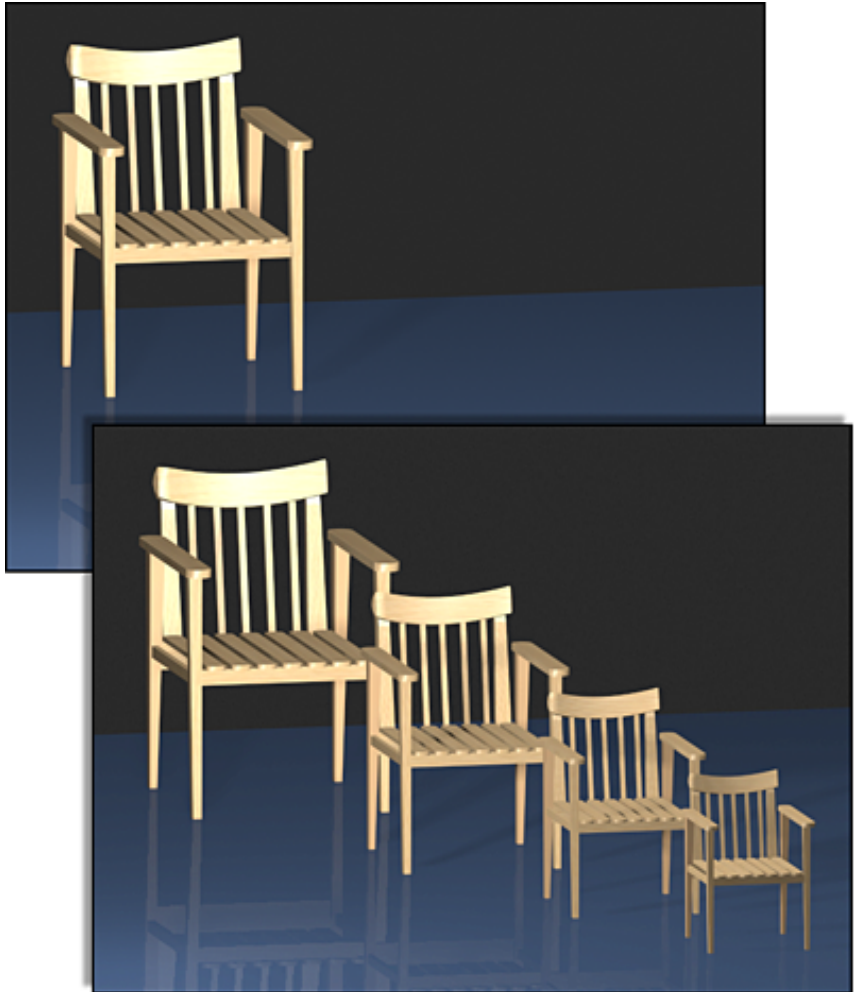
Linear array with progressive scaling
