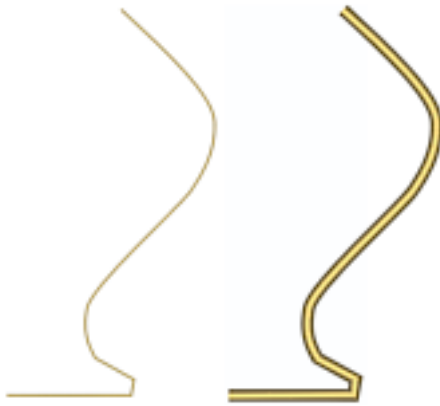
Splines rendered at thickness of 1.0 and 5.0, respectively
