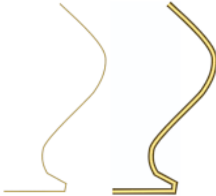
Splines rendered at thickness of 1.0 and 5.0, respectively
