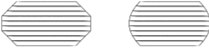
Bevels with linear and curved sides
