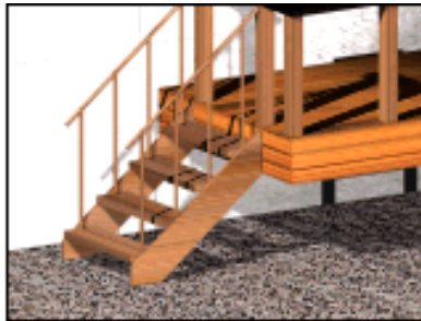
Left: The stringer extending below the floor. (Spring From Floor off.)
