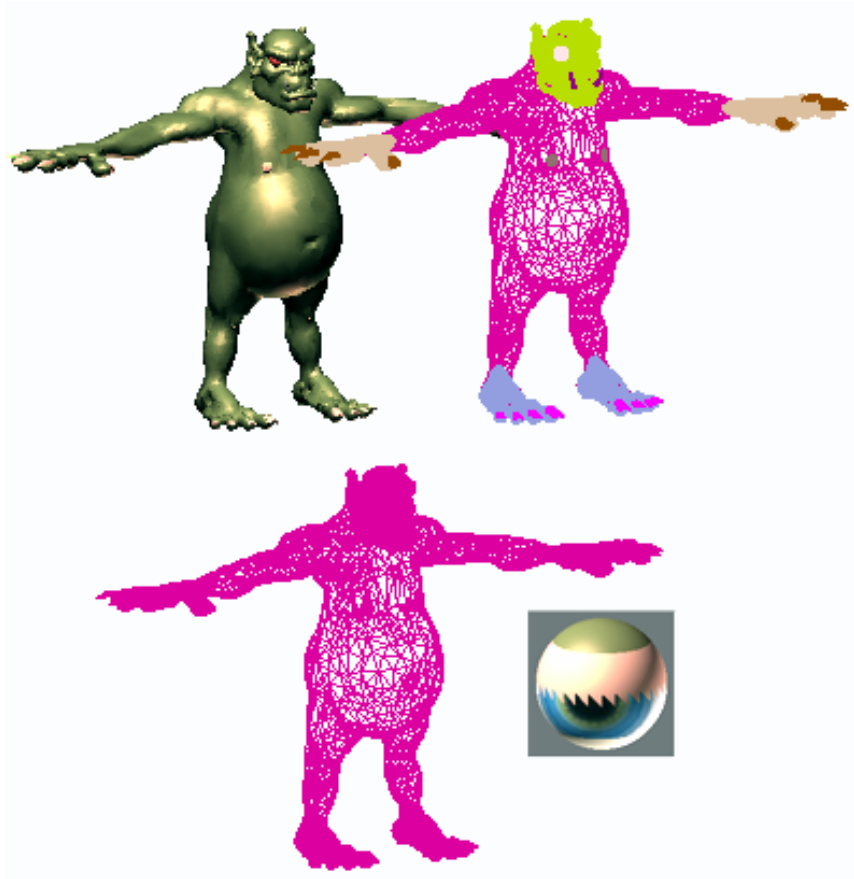
Shaded view of model (upper left); wireframe view of model (upper right); model with objects attached (lower left); and subsequent multi/sub-object material (lower right)
