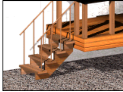
Left: The carriage springing from the floor. (Spring From Floor on.)
