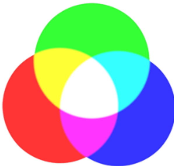
Additive mixing of colored lights
