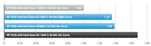
This chart compares two different HP Z420 Workstations with comparable HP Z400 Workstations which shows approximately 2 year old Intel technology so users can get an idea of the performance increase they might see by upgrading. Testing is based upon Cadalyst 5.4 Benchmark. All systems were tested with NVIDIA Quadro 2000 graphics, running Windows 7 Ultimate 64-bit operating system, 10k disk drives and Autodesk AutoCAD 2010. Tests were run January 2012 by HP Technical Marketing.
