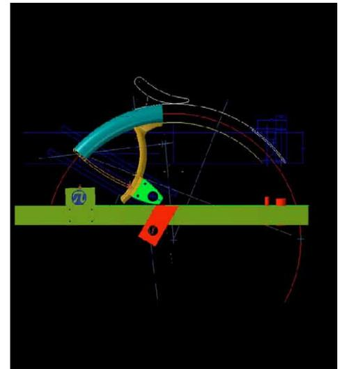
PiMoto aluminum monocoque in fixture drawing. Image courtesy of Pi Mobility.
