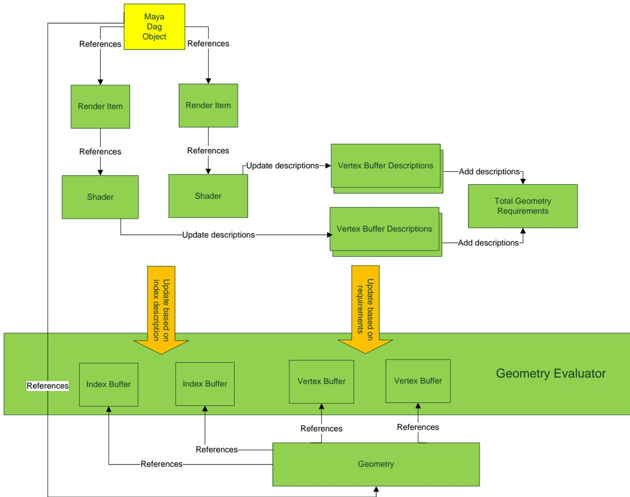
**Figure 8:** In this example, there is one dag object with two render items. Each render item has a shader instance associated with it. During shader evaluation, each shader instance will update its vertex buffer requirements (descriptions). When the geometry evaluator performs an update, it will update the vertex buffer and index buffers (per render item).
