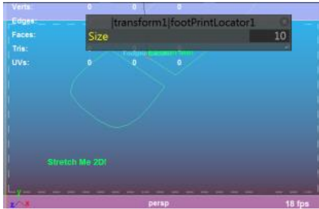
Figure 18: Snapshot shows the footprint manipulator. The “Stretch Me!” and “Stretch Me 2D!” UI are drawn using MUIDrawManager for the manip. The in-view editor is drawn for the plug-in internally. Note that it is layered to be on top of the footprint plug-in and spReticle UI, as well as the internal UI (polygon statistics shown here as an example).
