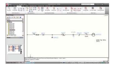
One-line component symbols can be related to parent/child counterparts on sche¬matic and panel layout drawings. Switch between one-line and all related components; when a component is modified, all related components update automatically.
