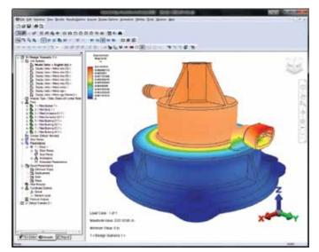
For products that use a fiber-filled material, export your Autodesk Algor Simulation model to Autodesk<sup>®</sup> Moldflow<sup>®</sup> Adviser or Autodesk<sup>®</sup> Moldflow<sup>®</sup> Insight software in order to simulate the plastic injection molding process and help predict the orientation of fibers in the manufactured part.
