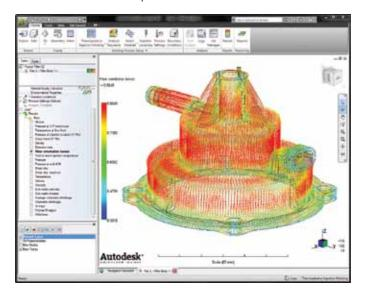
Within the Autodesk Moldflow software, calculate and view the orientation of fibers in an anisotropic resin and then determine the proper processing conditions to help optimize the structural properties in critical areas of the part.
