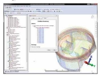
With the help of these tools, which group problems by type as well as by part and surface, you can quickly diagnose meshing problems and take corrective action to repair a mesh faster and obtain quicker, more accurate results.
