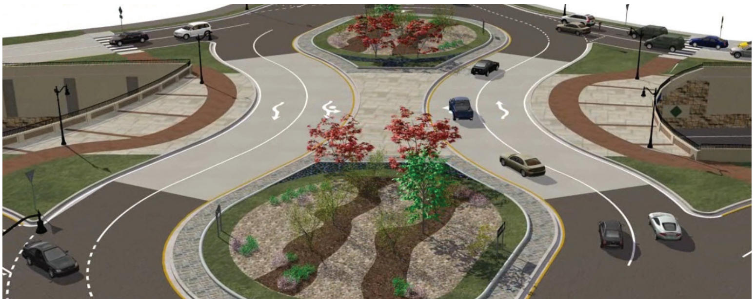
The redesigned Keystone Parkway in Carmel, Indiana, features the state’s first teardrop roundabout interchanges. Image courtesy of American Structurepoint, Inc.
