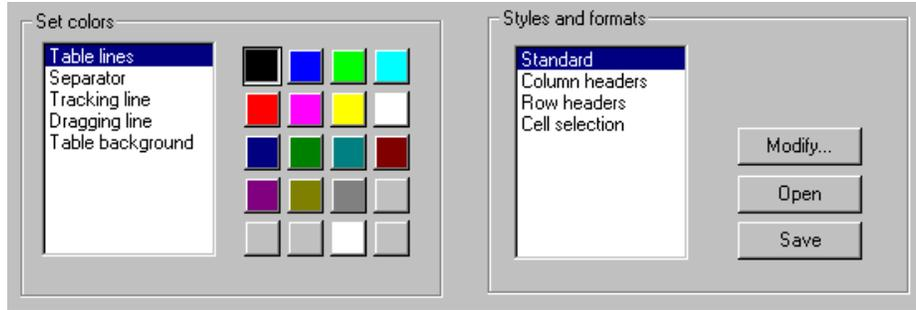
In the *Set colors* field the color of the following table elements may be chosen: table lines, separators, tracking lines, dragging lines and table background.
