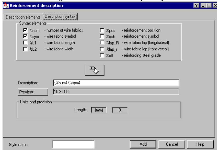
The options provided on this tab are used to define the description syntax of wire fabric distribution.
