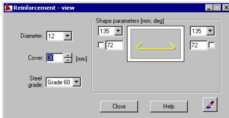
The following parameters of a reinforcing bar (longitudinal reinforcement) may be modified:
