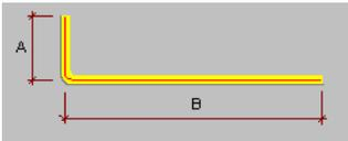
*Total along axis* - if selected, the length of a reinforcing bar is calculated - in reinforcement tables - as a sum of lengths of segments of the bar with hooks; lengths of bars along their axes are specified.
