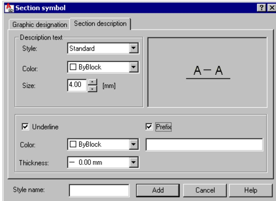
The options located in the *Description text* field concern the description of an RC element section. The following parameters can be set: font style, color and size. Below are two options:
