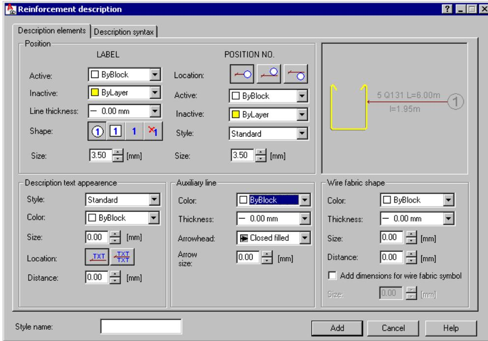
The first tab is used to define main settings (colors, line thickness, font size and style, etc.). Below are presented elements of a wire fabric description that can be defined by the user. The options included in the *Position* field refer to a label and to a number it contains (see the drawing below).
