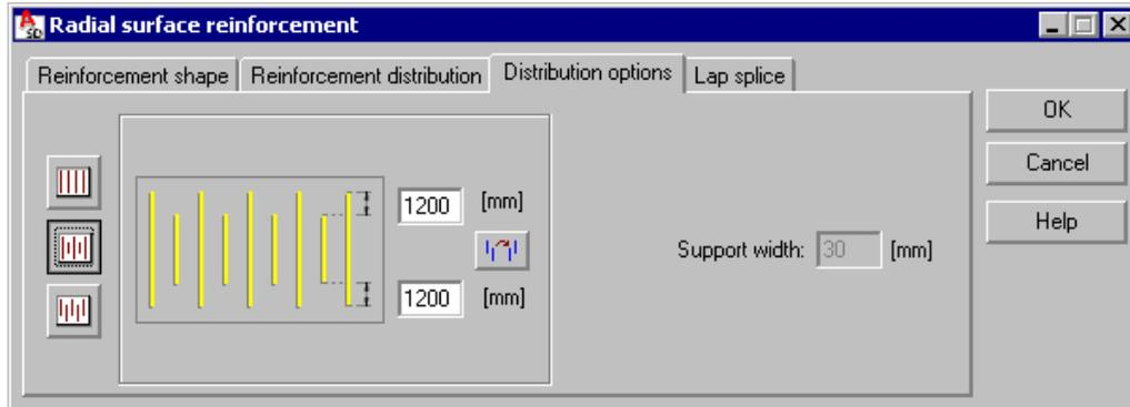
The options located on this tab enable more exact definition of the reinforcement distribution method; an arrangement for the entire distribution on the surface is defined here. The left part of the dialog box holds three icons:
