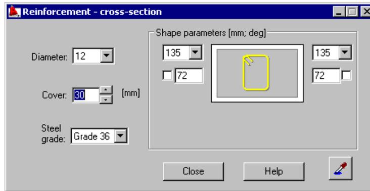
The following parameters of a reinforcing bar (transversal reinforcement) may be modified:
