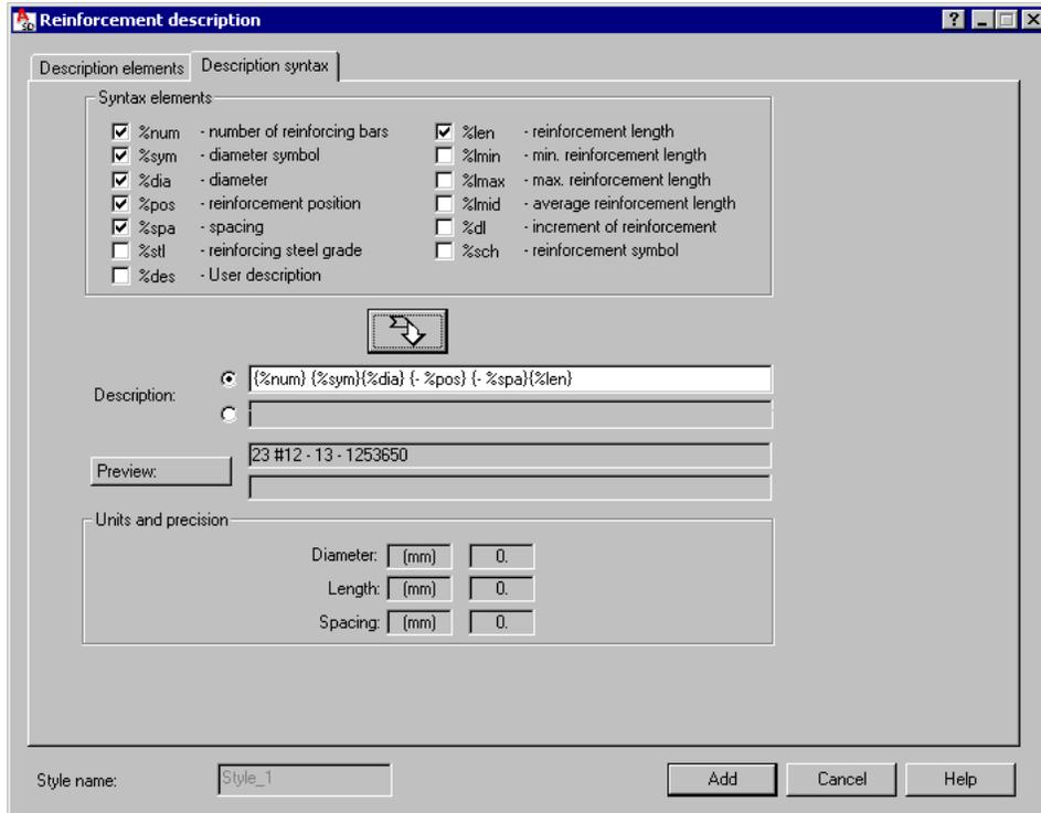
The options provided on this tab are used to define description syntax of reinforcement distribution.
