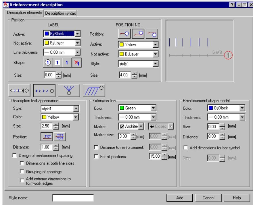
The options included in the *Position* field refer to a label together with a number the label contains (see the drawing below).
