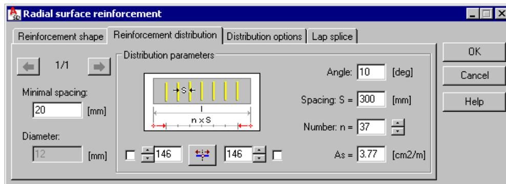
The options provided in the above dialog box are used for defining parameters of a reinforcement distribution.
