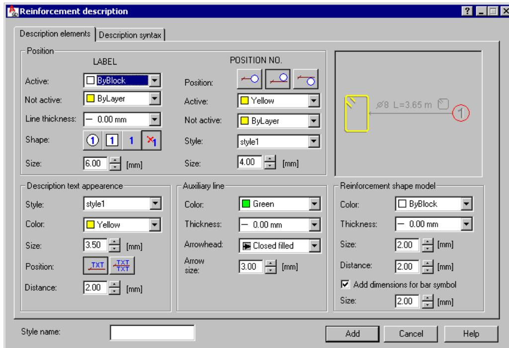
On the first tab main settings (colors, line thickness, size and shape of a font, etc.) are defined. The elements of reinforcement descriptions that can be defined by the user are discussed below. The options included in the *Position* field refer to a label together with a number the label contains (see the drawing below).
