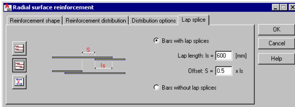
When distributing the main reinforcement, it may prove necessary to use reinforcement laps. If a reinforcement length exceeds the value defined in the preferences (e.g. 12 000 mm), then the options provided on this tab enable defining reinforcement laps (connections of reinforcing bars).
