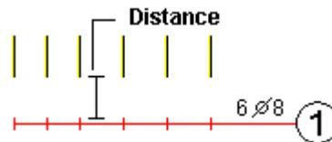
If the *For all positions* option is switched on, it means that the distance between the reinforcement description and the reinforcement distribution will equal the value defined for all positions.
