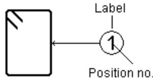
The first column of parameters pertains to a label and allows selecting color, line thickness, label shape and size. In the second column the user may define parameters of a number contained in a label: font style, color and size.
