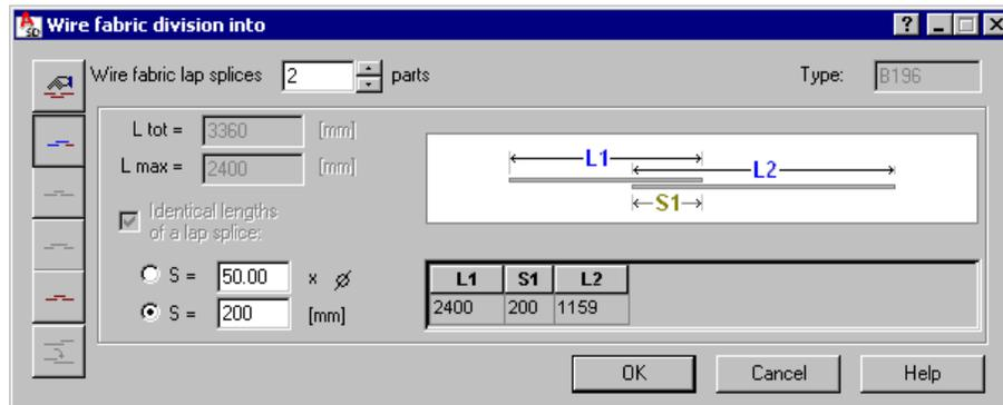
The left part of the dialog box contains the following icons determining methods of definition of a lap splice of a wire fabric:
