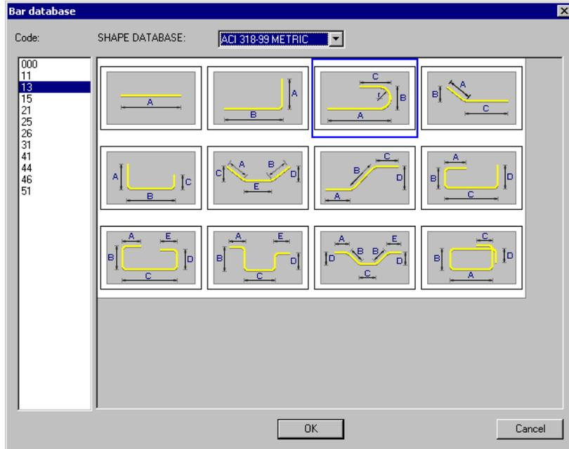
Definition of bars from the database consists in selecting one of them from the available shape list, and afterwards, defining successive bar segments by indicating next bar characteristic points presented in a schematic drawing (the user may also enter dimensions of individual segments from the keyboard).
