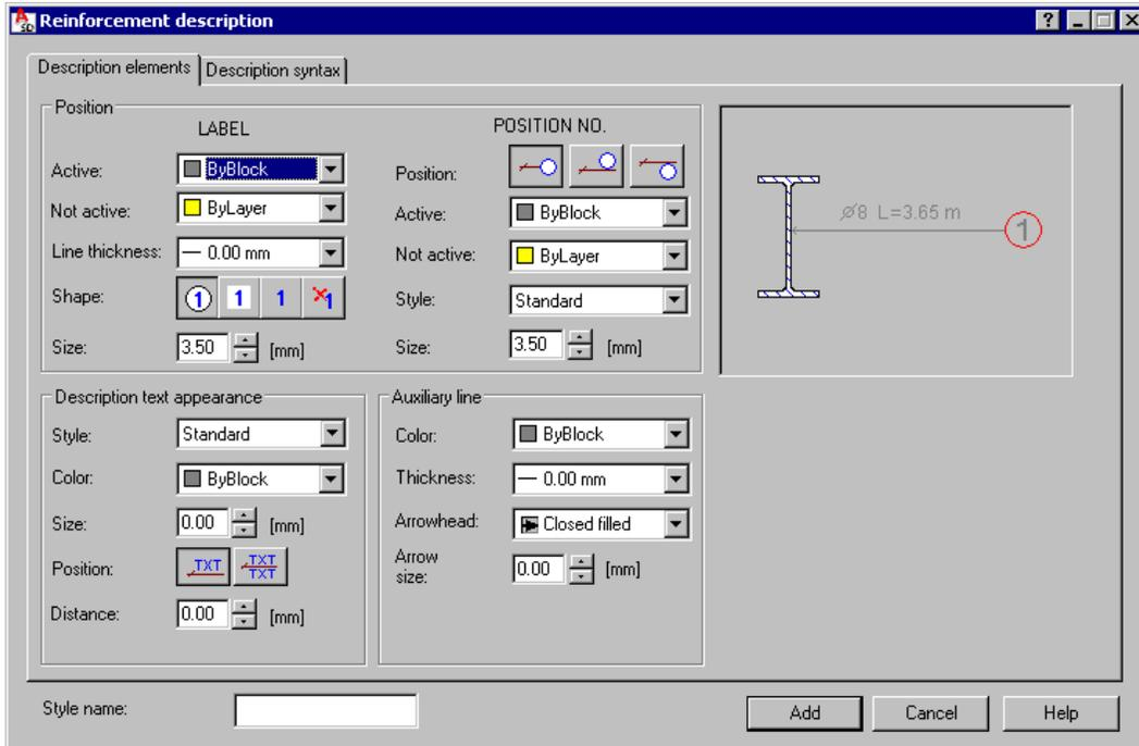
The first tab is used to define main settings (colors, line thickness, size and style of fonts, etc.). Below are presented elements of the steel profile description that can be defined by the user. Options in the *Position* field refer to a label and a number in the label (see the drawing below).
