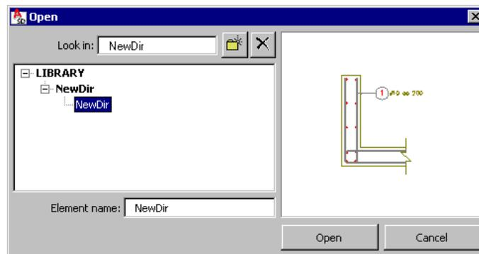
After selecting a linear element saved earlier on the disk, a block of drawing elements is placed in a drawing. The linear element chosen is assigned name and length; the spacing of elements over the length (e.g. 3 meters of length with spacing every 20 cm) is also specified.
