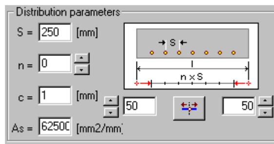
The left part of the above dialog box contains the parameters controlling reinforcement distribution within one zone:
