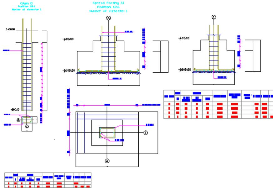
The first stage of drawing generation is to create views in the model space. To create views for projections of the spread footing and the column, do as follows:
