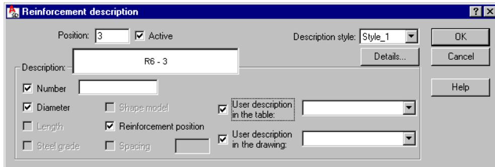
The options provided in this dialog box enable final selection of the reinforcement description. It can be performed by switching off active variables initialized based on the syntax defined.
