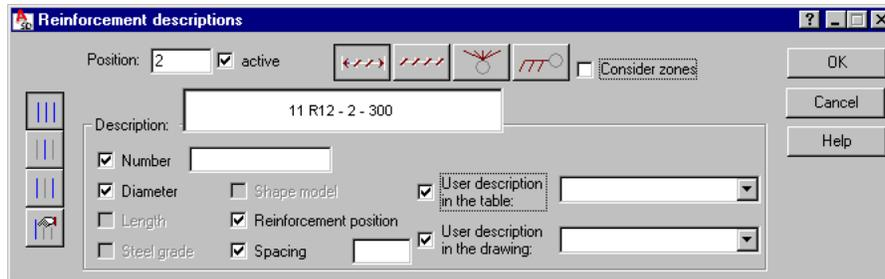
The options included in this dialog box enable final selection of reinforcement description and distribution. It may be done by switching off active variables initialized based on the defined syntax.
