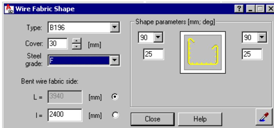
The following parameters of a wire fabric in the cross section can be modified:
