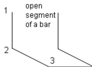
cover – determines a cover value for individual segments of reinforcement
