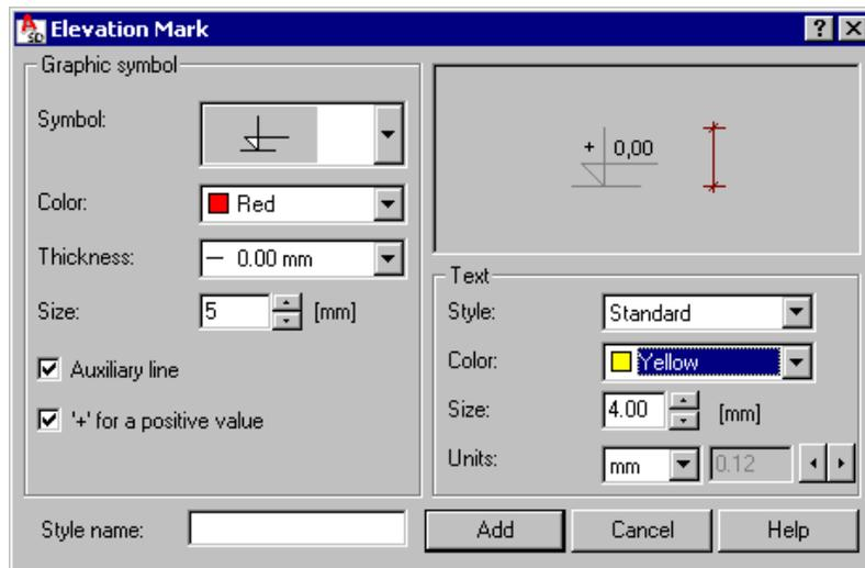
The *Graphic symbol* field holds parameters of a symbol representing a level in the drawing: symbol type, color, size and thickness of the line in the symbol. Below are two options:
