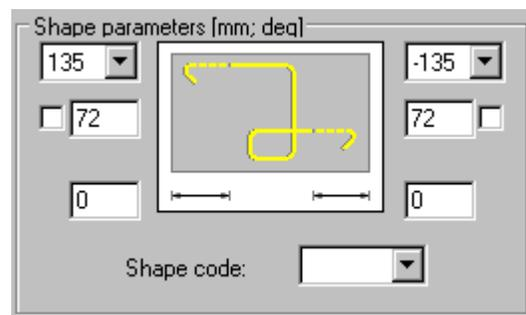
This dialog box allows defining any shape of reinforcement.
