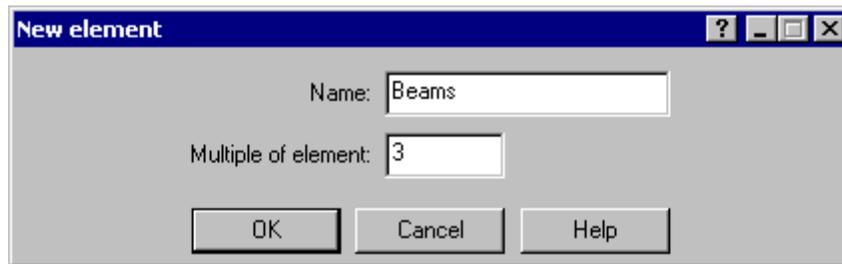
In the above dialog box the user should specify a name of the element and a number of these elements (multiple of element); After pressing the **OK** button, indicate in the drawing the objects that should belong to the element being created; it is possible to select contours (e.g. beams along with axes, section symbols, an elevation mark) and reinforcing bars. If reinforcing bars have not been drawn in a formwork yet, then only formwork parts will be included in the defined element.
