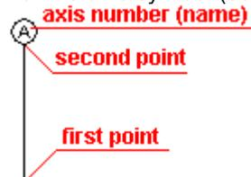
The axis number is proposed according to the settings in the default style; while inserting the axis any number may be typed (every next one will be inserted according to the recently-applied numbering). The axis number may be modified using the context menu option.
