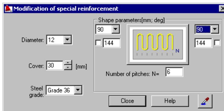
The following parameters of a reinforcing bar (special reinforcement) can be modified:
