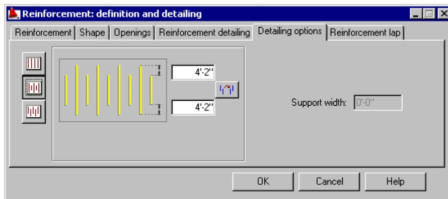
The options located on this tab enable more exact definition of the method of reinforcement distribution; here the array valid for the entire distribution on the surface is defined. In the left part of the dialog box three icons are provided:
