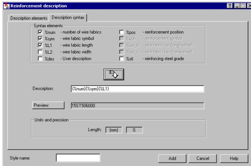
The options on this tab are used to define a description syntax for a wire fabric symbol.
