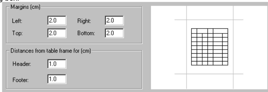
The above dialog box allows determining (identically as in each text editor) page margins: left, right, top and bottom. Moreover, the user may define distances between the table frame and header or footer.
