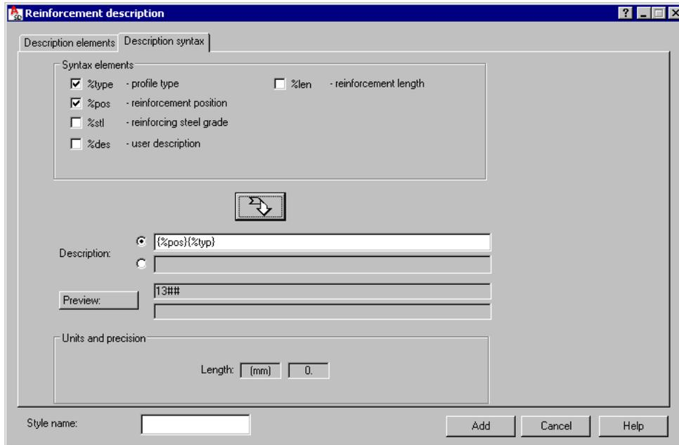
Options on this tab are used to define a syntax of the steel profile description.
