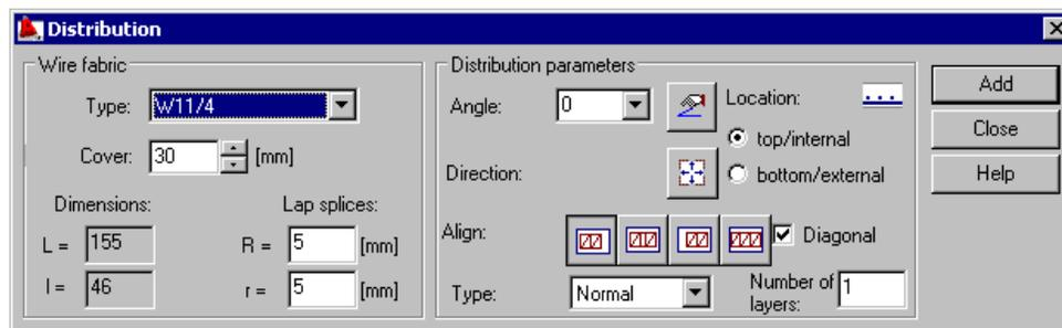
The options contained in the dialog box are used to parametrize distribution in the region defined:
