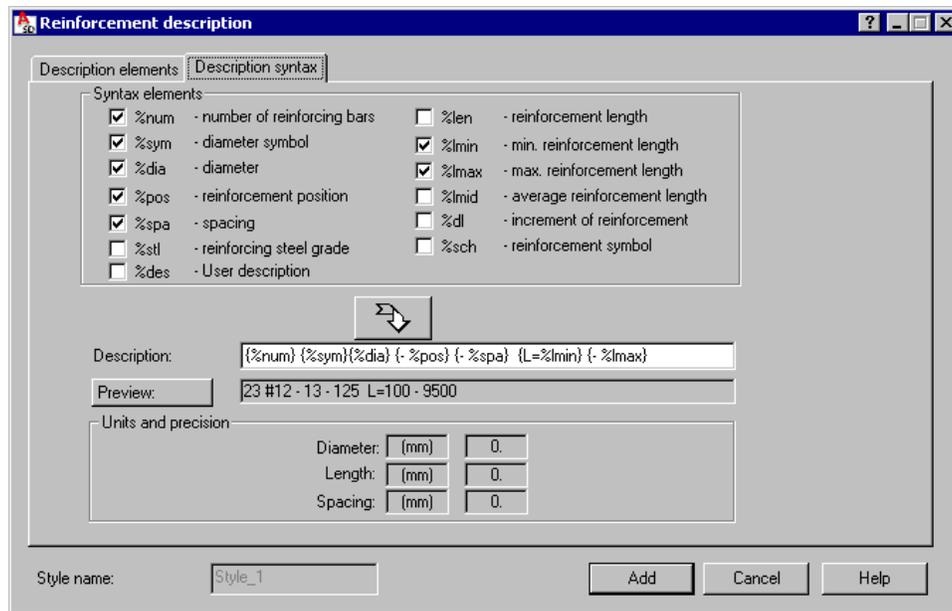
The options provided on this tab are used to define description syntax for a symbol of reinforcement whose description is provided outside the formwork contour.
