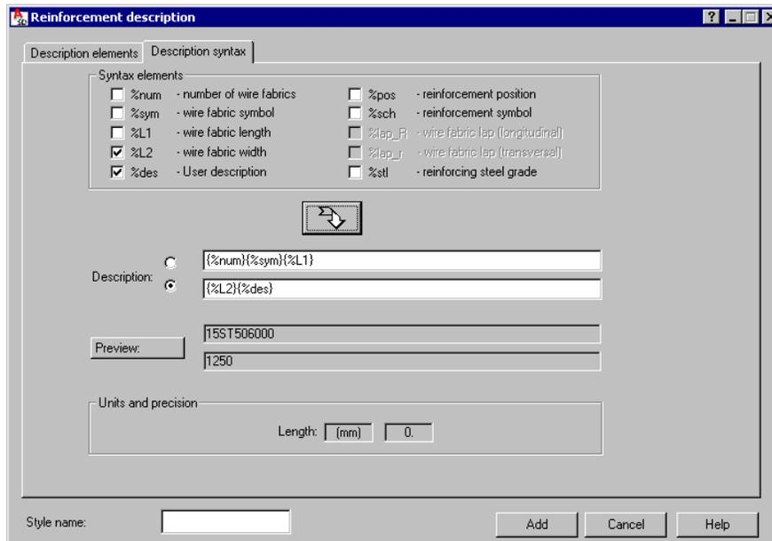
The options provided on this tab are used to define a syntax of a description of a wire fabric shape.
