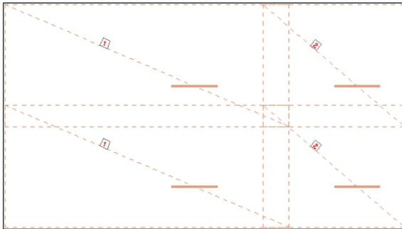
passing and half-way types - wire fabrics are shifted in relation to each other by half the length (to avoid concentration of lap splices of several wire fabrics at the same point) – see the drawings below
