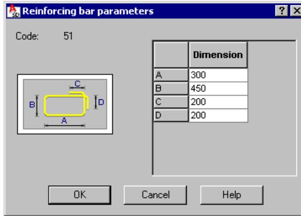
The above dialog box contains a table that displays dimensions of bar segments. The field with a shape code is filled out automatically depending on a typical shape selected. Both modes of reinforcement definition are synchronized with each other. It means that both definition modes can be used alternately.
