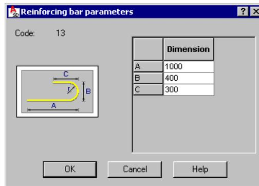
The above dialog box contains a table that displays dimensions of bar segments. If the dialog box is opened while a bar is being defined, then dimensions that are not defined yet will be assigned zero value. The user will be able then to change the bar segment lengths determined and to complete the dimensions missing.
