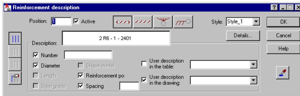
The options provided in this dialog box enable final selection of reinforcement description and distribution. It can be performed by switching off active variables initialized based on the syntax defined.
