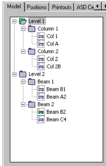
Individual components included on the list presented on the *Model* tab may be freely composed: deleted, shifted between folders - using the mouse; all these operations will result in updating the data contained in the **Element manager** dialog box.
