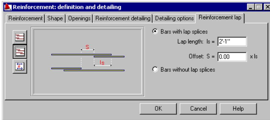
When main reinforcement is being distributed, it may prove necessary to use reinforcement laps. If reinforcement length exceeds the value defined in the preferences (e.g. 12 000 mm), then the options provided on this tab enable defining reinforcement laps (connections of reinforcing bars).
