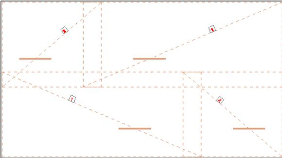
There is also a possibility of simplified presentation of wire fabrics; the drawing below shows the simplified method of presenting a generated wire fabric.
