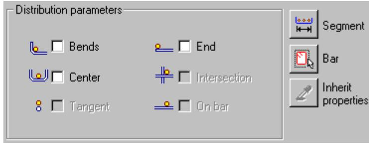
NOTE: The options: bar intersection, tangent to bar and on bar are not accessible in the current program version.
