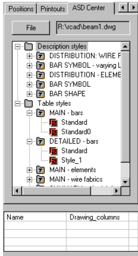
After pressing the **File** button and selecting a file with an earlier-saved project, the *Inspector* dialog box shows all the defined styles that may be used in the current project. After highlighting a selected style, pressing the right mouse button and choosing the *Add* command, the selected style is added to the styles available in the current project.
