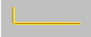
*Real* – if selected, then in tables the reinforcing bar length will be determined as exact length of bar axis
