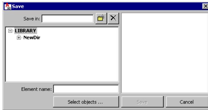
After pressing the **Select objects** button, an element (a block of drawing elements) should be pointed on the screen. Such an element may be saved to the database.
