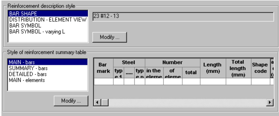
The dialog box provides basic information about the styles currently defined and relevant reinforcement or table to which these styles apply.
