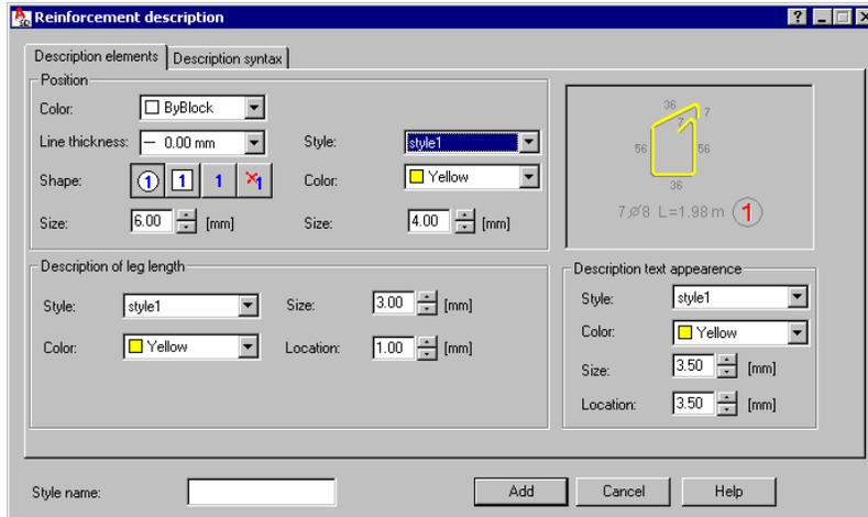
The options included in the *Position* field refer to a label together with a number the label contains (see the drawing below).
