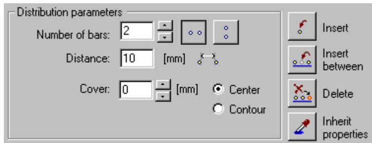
The distribution method is intended for all these cases where standard methods of reinforcement distribution prove ineffective. This method will allow the user to position a bar or a bar group freely, based on the distribution carried out earlier; the distribution may also be defined independently.
