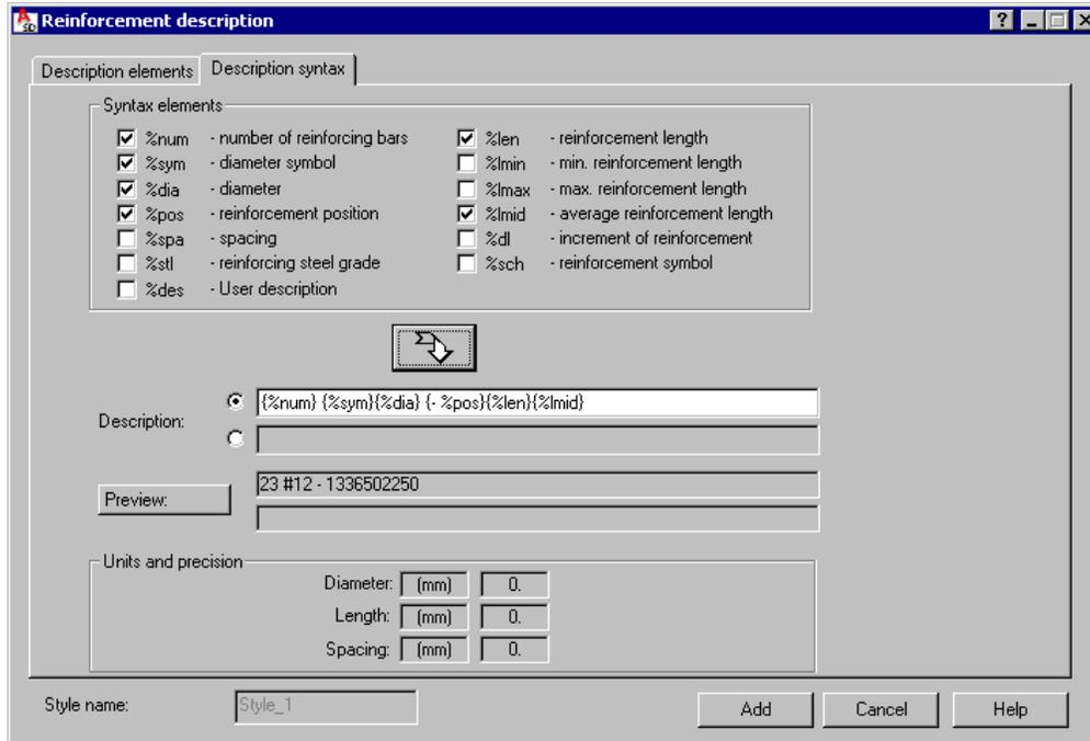
The options provided on this tab are used to define syntax of a reinforcement description; The above dialog box provides access to both the defined general style of reinforcement description and to the mechanism allowing free composition of syntax and contents of reinforcement description.
