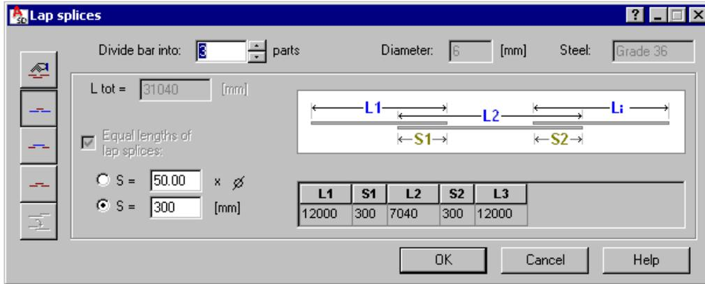
The left part of the dialog box comprises the following icons determining methods of lap splice definition:
