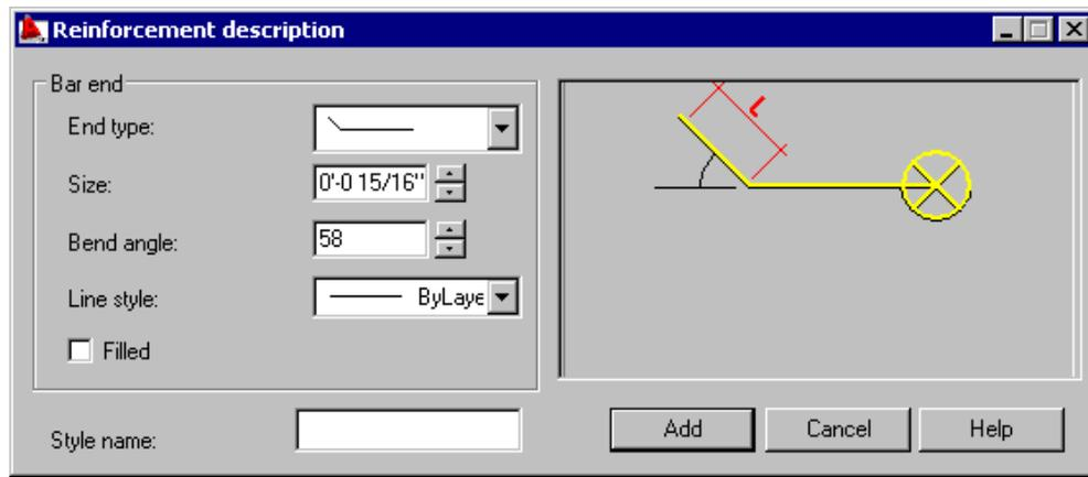
The *Bar end* field has options for presenting reinforcing bar ends (additional lines at bar ends) in distributions. These lines are additional objects connected with the bar.
