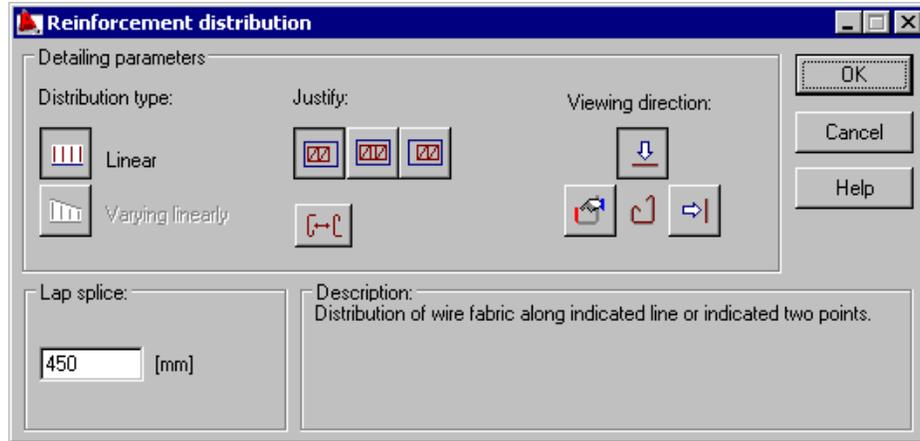
The options in the left part of the dialog box, in the *Detailing parameters* field, allow determining a type of reinforcement distribution:
