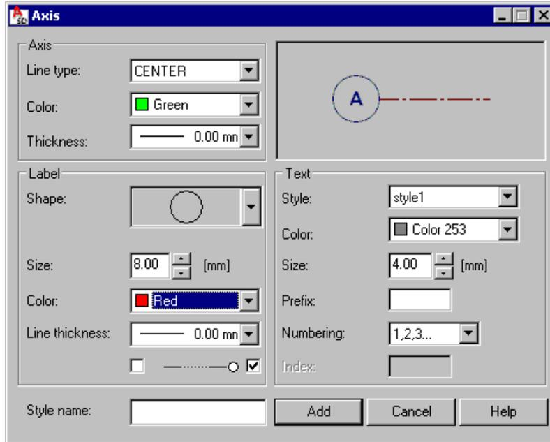
The *Axis* field holds parameters of a line presenting the axis in a drawing: line type, color and thickness.
