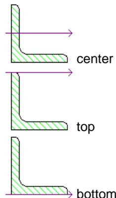
it is also possible to define an offset (shift) of the point of insertion of a steel profile; the offset denotes a shift of the profile center with respect to the insertion axis. an offset value may be positive (offset upwards) or negative (offset downwards)
