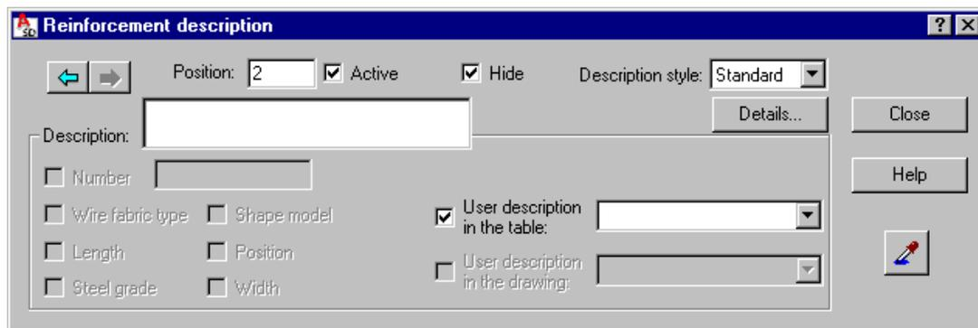
The options in this dialog box enable final selection of a reinforcement description. It can be achieved by switching off active variables initialized on the basis of a defined syntax.
