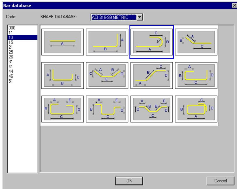
Definition of bars from the database consists in selecting one of them from the available shape list, and afterwards, defining next bar segments by indicating next bar characteristic points presented in a schematic drawing (the user may also enter dimensions of individual segments from the keyboard).
