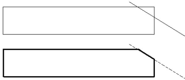
Cutting the profile is possible by specifying positions of two points that define a line. Additionally, a direction is indicated (a point on one side of the cutting line): it determines on object part to be cut off.
