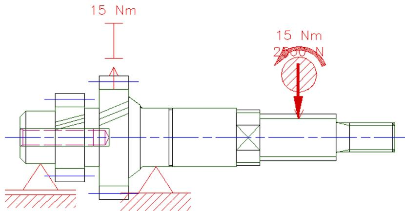
All boundary conditions necessary for a shaft calculation are specified.
