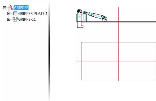
Once one view of an xref component is inserted, the other views can be inserted as normal.
