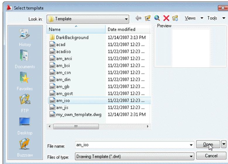
This creates a new drawing based on the am\_iso template. Use Save As to save the drawing file with an appropriate name.
