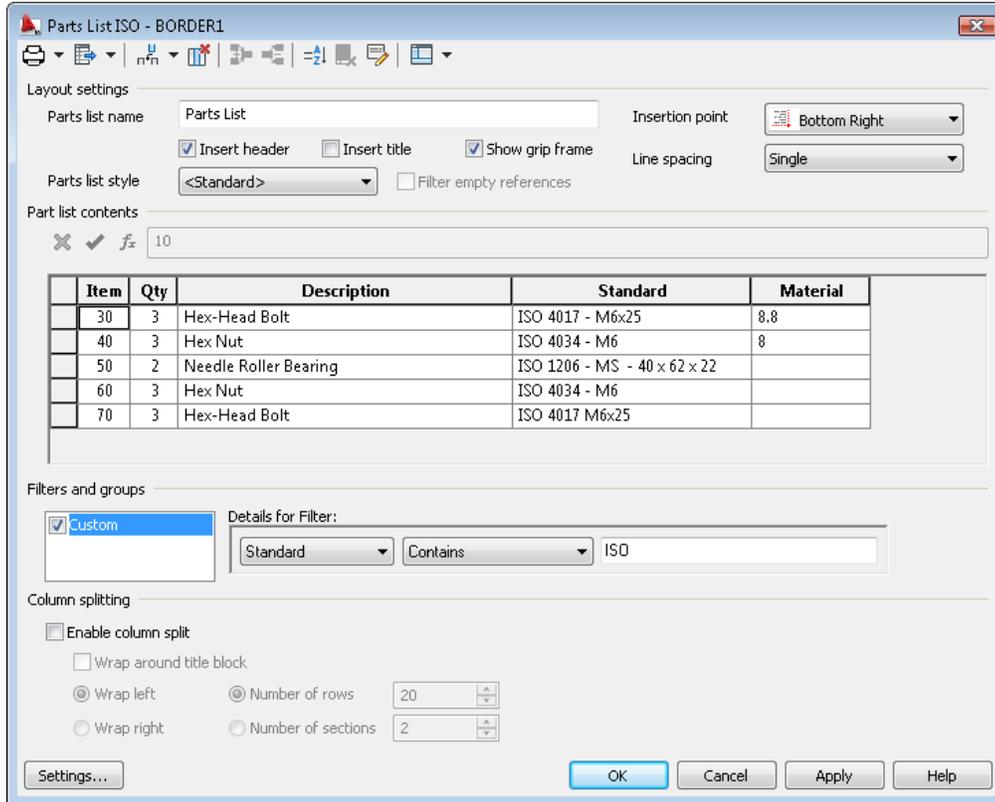
The filtered parts list is displayed in the drawing. The defined filters are saved with the parts list and can be used again later.
