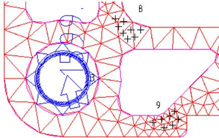
The mesh is refined at the specified points.
