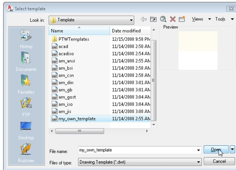
Start the new drawing using the settings of the previously saved template.
