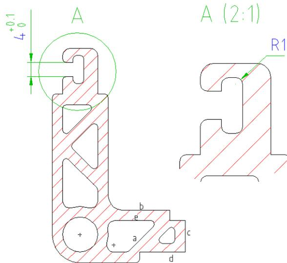
The Power Dimensioning command recognizes the different scale area. If you dimensioned the radius in the original drawing, the dimension value would be the same. The text height is also the same, as per the selected drafting standard.
