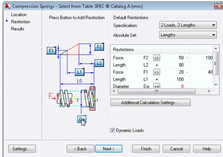
A row for specifying the outer diameter  $D_a$  is added to the restrictions table.
