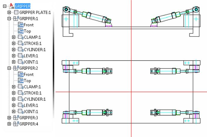
Next, you assemble the components under an assembly, named GRIPPER ASSEMBLY.
