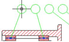
Because the balloons are numbered automatically, depending on where you located the part references, the appearance of your drawing can be different.
