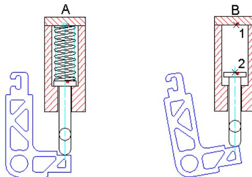
The spring is copied into view B in its compressed length.
