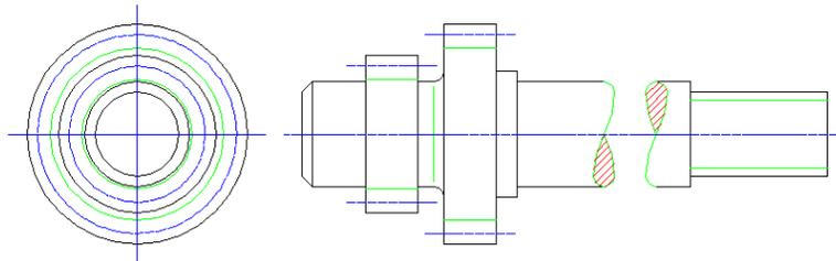
In the mechanical browser, the new right side view is listed within the shaft component along with the existing front view. The right side view includes its hide situations.
