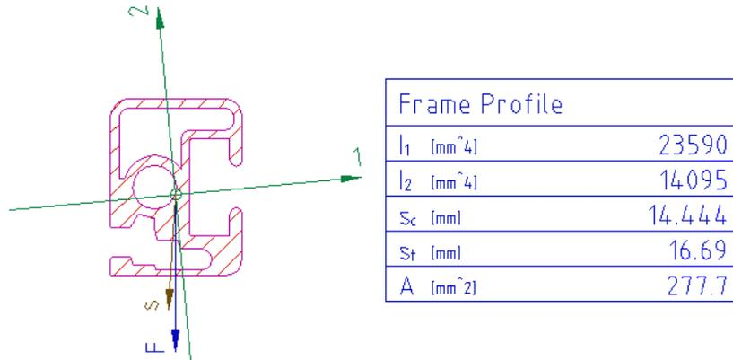
**NOTE** The main axes, 1 and 2, are the axes with the most and least deflection. The F arrow displays the direction of the force, the s arrow displays the resultant deflection. The moment of inertia block shows the moments related to the main axis, the maximum distances from the edges, and the calculated area. For more detailed information, see Help.
