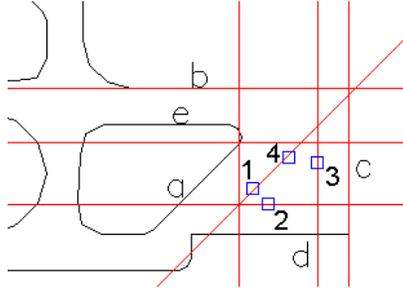
All construction lines have been inserted, and the contour can be generated.
