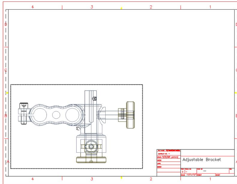
The base view is placed in the lower-left corner of the drawing.
