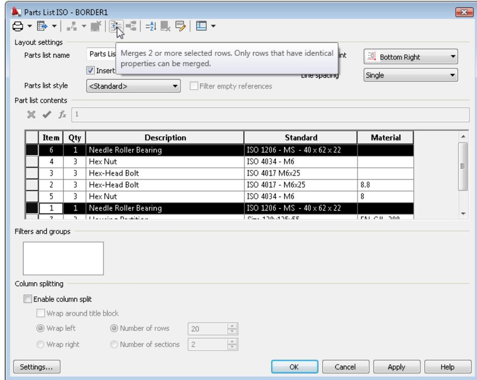
The two rows are merged. In the Parts List dialog box, Item 6 now has a quantity of 2, and item 1 is missing.
