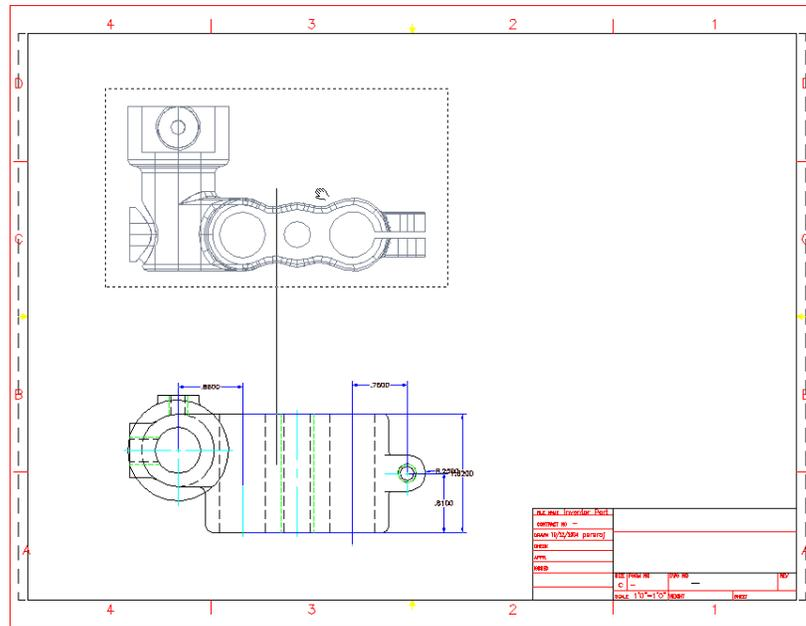
The view is placed in the upper-left corner of the drawing. Parametric dimensions read from the Autodesk Inventor part are displayed
