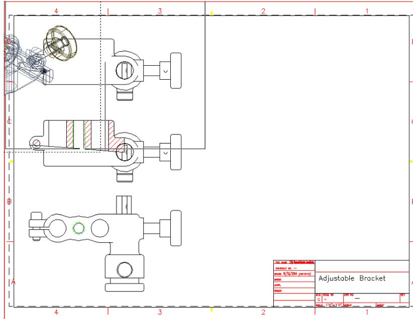
**NOTE** The details shown in the view that is generated depend on where you place the view. When you drag to the left, the isometric view that is generated reveals a hole and a screw. They would not be visible if you placed the view elsewhere.
