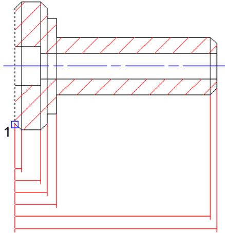
Starting point for next extension line: *Press ENTER to end the command*
