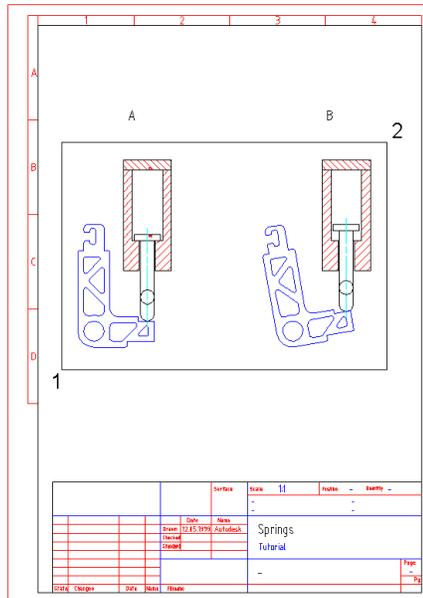
The drawing shows two views (A and B) of the lever and spring housing, to reflect two different states of compression.
