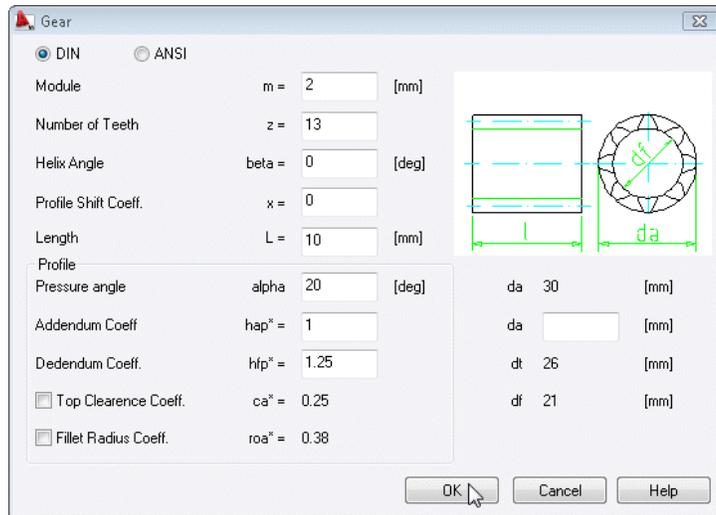
**NOTE** Here, the DIN standard requires that you indicate the module. The ANSI standard requires the Diametral Pitch  $1/\text{module}$ . You can switch between these two representations using the DIN and ANSI options.
