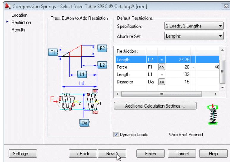
The possible springs are calculated and the results are displayed in the Compression Springs - Select from Tables SPEC® Catalog A [mm] dialog box.
