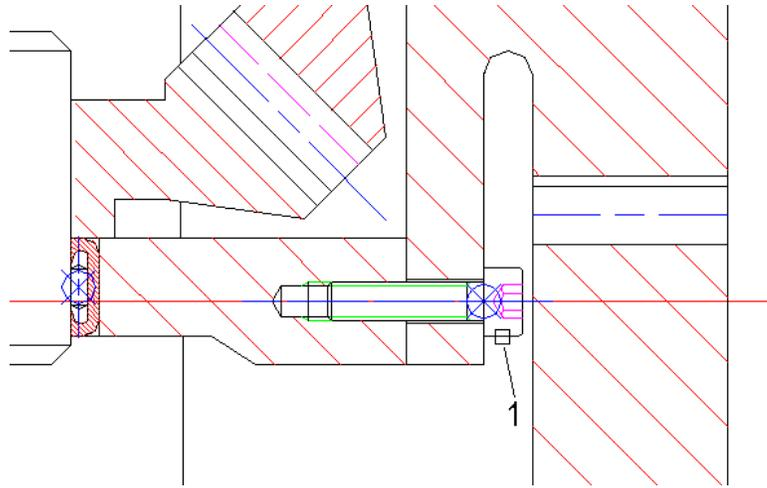
The screw connection is deleted and the lines and hatch are restored.
