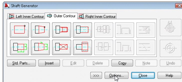
**4** In the Shaft Generator - Configuration dialog box, specify:For Segment inserted: **Insert**Stationary Shaft End: **Left**Adjust Centerline: **Yes**Front View: **Radius Reflection Line, Check contour**Side and Sectional Views: **Sectional with Background, Always update**View of Interrupt: **Hatch**If shaft is in background, hide standard part too: **Yes**
