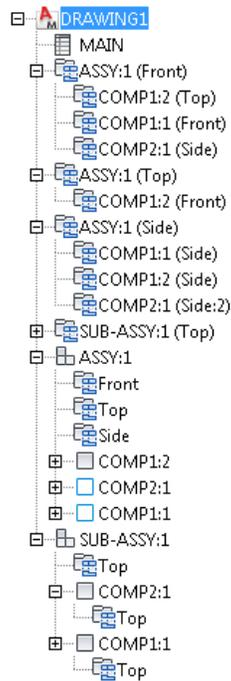
Note that the component SUB-ASSY is already created (1) and COMP1:1 and COMP2:1 are components of it. Also, the COMP1:1 and COMP2:1 continue to exist as components of ASSY1 (2), but the icon changed. This icon indicates that the component is a *Ghost Component*. Ghost components are containers of the views of components that are in an intermediate state of restructure.
