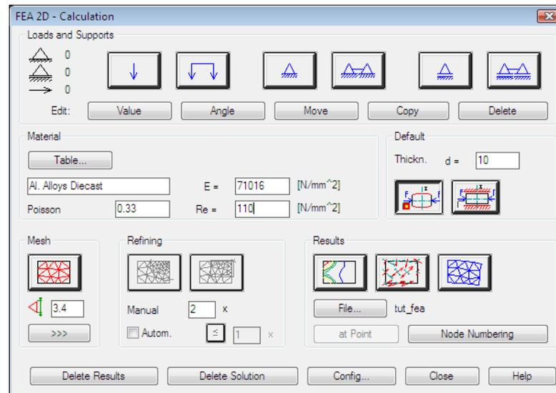
Select the thickness and the material of the lever.
