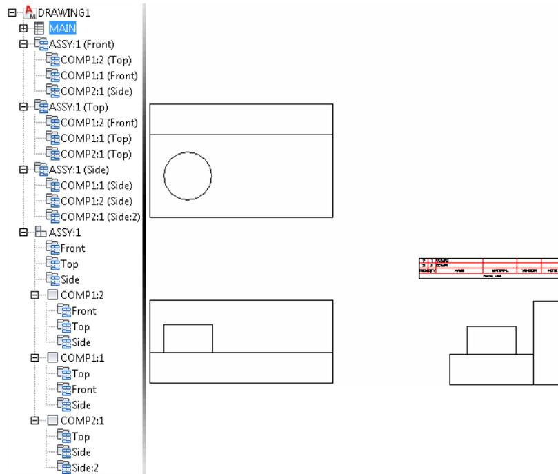
By associating views through a single component, the BOM is managed accurately and semi-automatically. You can manage component attributes through the BOM editor or directly on the component from the Mechanical Browser.
