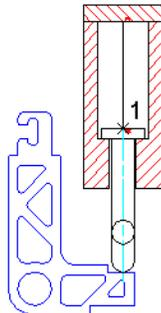
Use view B of the lever and spring housing to define the compressed spring length.
