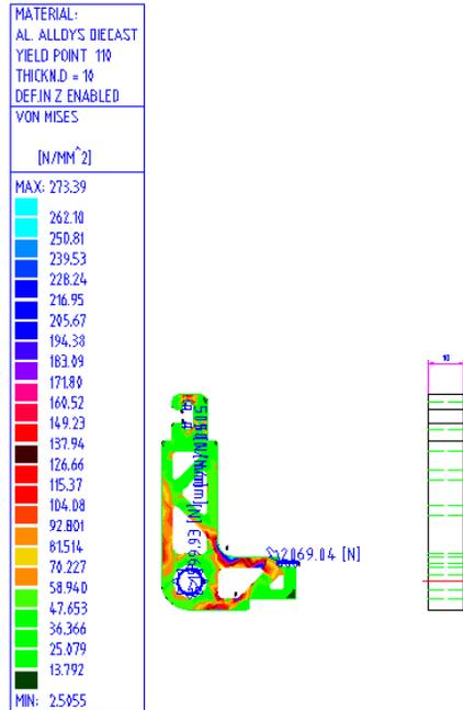
After calculation, the support forces are displayed near the support symbol.
