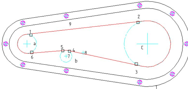
The tangent definition is finished, and the length of the chain is calculated. Because the length is divided into whole numbers of links, one sprocket has to be moved to achieve such a length.
