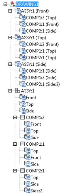
In this view, the Mechanical Browser shows the hierarchy of components, component views as well as indicates which component owns a given component view. In practice, you can work with the view settings that makes most sense to you.
