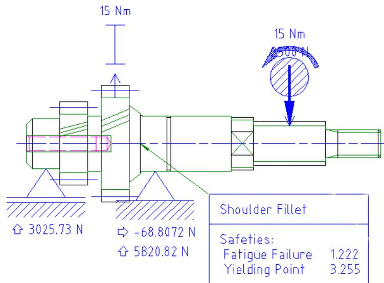
The safety factors are greater than 1.0, so the shaft does not need to be redesigned at this notch.
