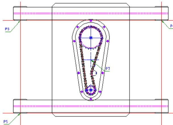
Define the 2D hide situation for the girder assembly and the chain drive.
