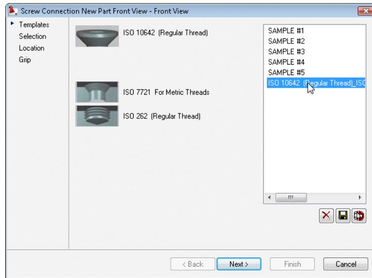
The Screw Connection New Part Front View - Front View dialog box contains the screw connection as it has been stored in the template.
