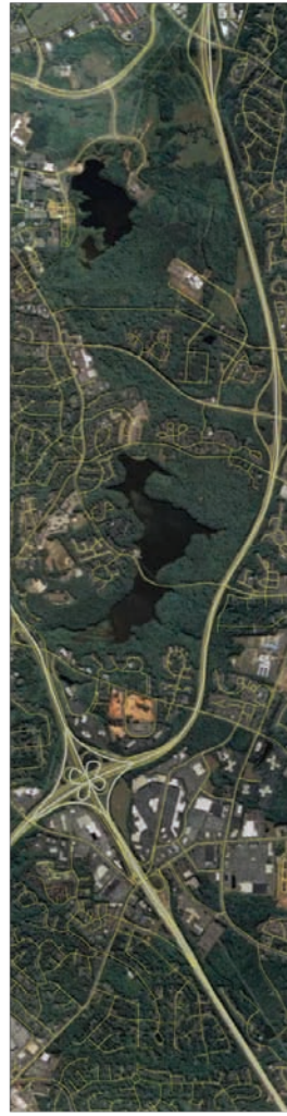
This color image was exported from Google Earth and saved in a geotiff format. It was then brought into AutoCAD Map 3D to match the scale and position of the existing road features in AutoCAD Map 3D.
