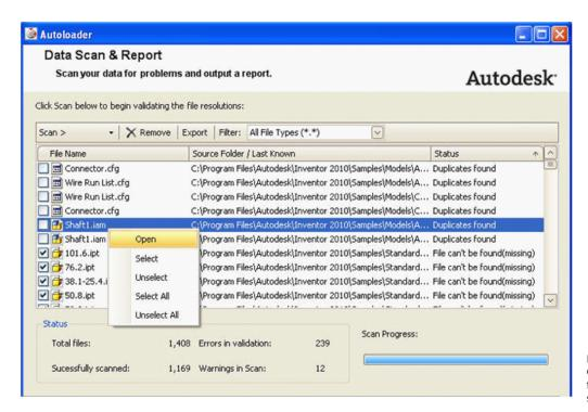
Note: As of Autoloader 2010, it is possible to open CAD files directly from the scan dialog. To open files from the Autoloader, select the file, right click, and select Open.
