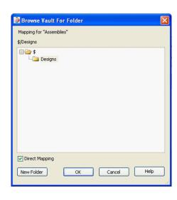
Traditional folder mapping to the parent folder (Direct Mapping not selected) would result in the following where the new Assemblies folder is created under the default Designs top level folder:
