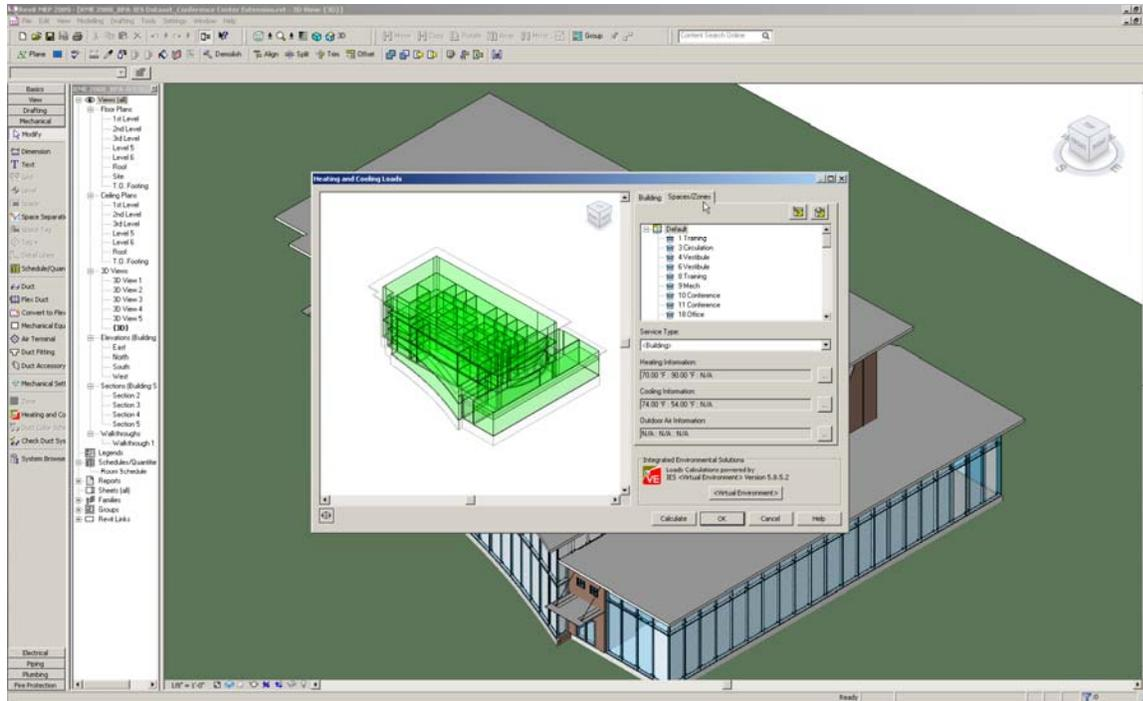
*BIM and its reliance on a digital building model streamlines the design and analysis functions, allowing designers to quickly evaluate design alternatives and make better decisions to iterate on a greener design.*
