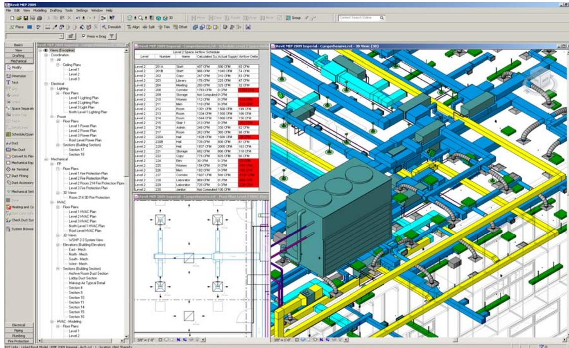
*State-of-the-art BIM software uses a centralized, parametric model—where all the plans and sections, the quantity takeoffs, and other related documentation are “live” views of the model and are automatically coordinated by the software—resulting in better coordinated construction documents that minimize errors and omissions.*
