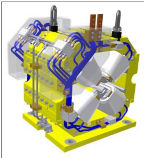
Rendering of storage ring quadrupole magnet.
