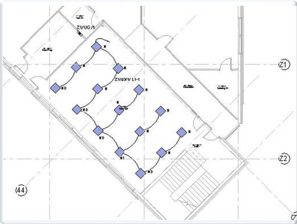
Figure 6. Buro Happold uses Revit MEP to create lighting layouts such as the one shown here.
