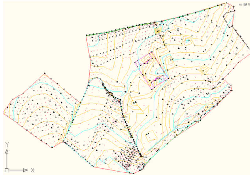
Figure 6: Surface created from breaklines and point groups with specified contour style
