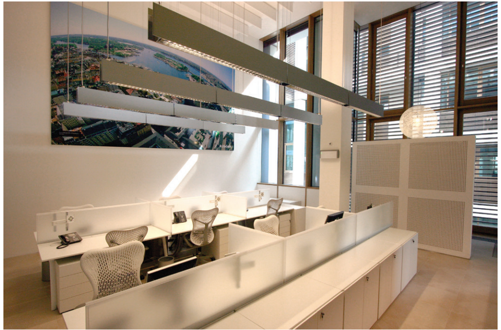
The office includes an energy-efficient lighting system with daylight sensors. Image courtesy of Goring & Straja Architects.
