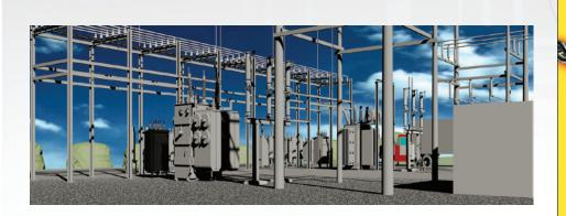
It can be difficult for even the most experienced people to visualize the whole project, working only from lines on multiple design sheets – and that's what you get with 2D tools. The new 3D model-based design approach will allow construction crews to explore the big picture and the smallest detail of the design. This will help them to plan their work more efficiently and avoid rework due to misunderstanding some aspect of the design.
