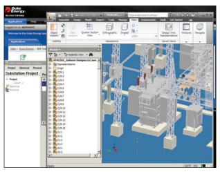
In a sense, they build a digital prototype of each substation before it's built. If a beam is impeding access to equipment, they see it immediately, and they can take steps to improve access. Duke Energy believes that 3D modeling has the potential to help enable better and more sustainable design. With 3D modeling, the designer will be able to easily explore how changes might improve substations or could lead to minimized waste and rework during construction.
