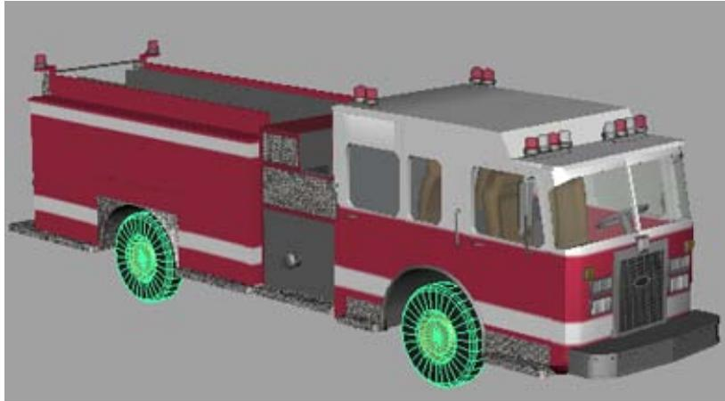
Unlike the doors, a fire truck's wheels are expected to move together. For example, the wheels on the front and back axles should spin together, and the front wheels should turn together. To do this, you need to create a custom attribute to control both components at once. Then you can publish your custom attribute to the asset.
