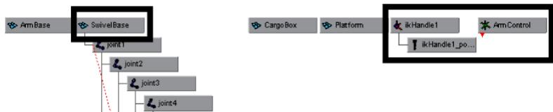
ArmControl and IK Handle are not parented into the SwivelBase hierarchy. Because ArmControl and IK Handle control the movements of the mechanical
