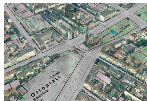
Figure 2: Create more informative city models by combining scanned maps with detailed building models.
