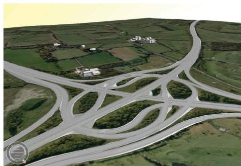
Figure 4: Combine GIS data prepared in AutoCAD Map 3D software and roads designed in AutoCAD® Civil 3D® software to better visualize a proposed highway interchange.
