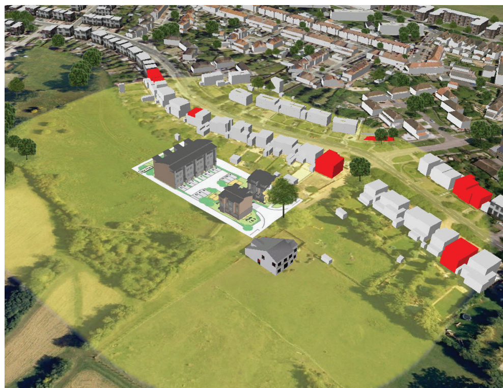
Figure 1: Incorporate detailed 3D building models along with data prepared in AutoCAD® Map3D software into your city model to better illustrate affected residential buildings within 100 meters of a proposed development.
