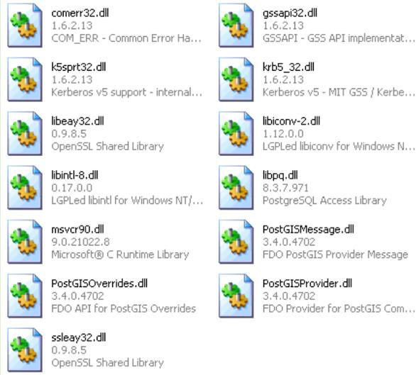
Copy and paste the DLLs listed below into C:\Program Files\AutoCAD Map 3D 2010\FDO\bin and update the providers.xml file to register the PostGIS FDO Provider.
