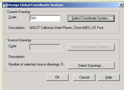
Assign CA-I or proper coordinate system to Map 3D.
