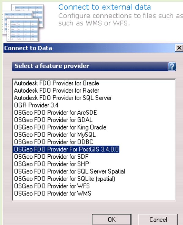
Start MapGuide Studio and click Connect to External Data. Now you should see the PostGIS Provider listed with the other providers available. You can see all the OSGEO providers can be configured with AutoCAD Map 3D as well as with Autodesk MapGuide Enterprise with this common process.
