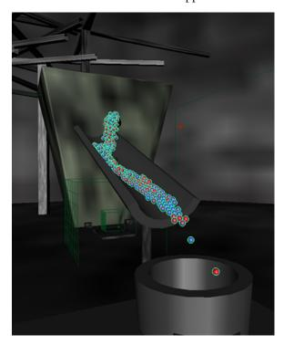
If the problem with particles escaping persists after you turn down the **Bounce**, you can use either **Friction** or **Stickiness** to further stabilize the particles on the chute.
