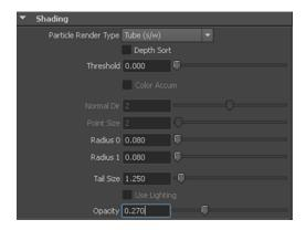
For more information about **Tube (s/w)** type particles, see *Particle nodes* in the *Dynamics* guide of the Maya Help.
