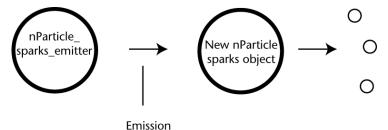
To ensure that sparks are emitted in locations and at times that appear random. and in the correct amount, you need to control the number of nParticle\_sparks\_emitter particles. To do this, you use the **Emission Overlap Pruning** attribute to emit particles at specific areas along the chute. The result is an effect of randomization without the use of a particle expression or scripting.
