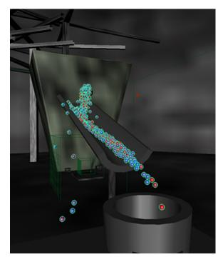
Since you will later convert the nParticles to an output mesh, you want to ensure that no particles move too far away from the location of the nParticle mass as this enlarges the bounding box area of the resulting mesh. The **Output MeshMax Triangle Resolution** defines the area of the mesh bounding box.
