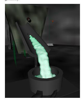
Also notice that generating an nParticle mesh slows down the simulation. In particular, low **Mesh Triangle Size** values and **Mesh Smoothing Iterations** greater than 3 can quickly slow simulation time and decrease overall performance. However, both settings increase the quality of the mesh. For larger simulations involving output meshes, caching the nParticles can decrease simulation time.
