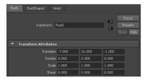
The **Translate** values position the fluid container at the top of the slag chute. You can now add the emitter to the fluid container.
