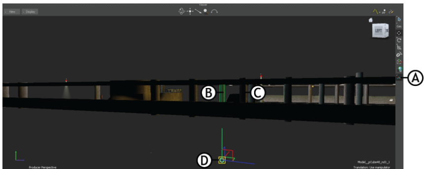
Parking lot scene rotated to locate the pivot of pillar C A. Pivot Mode B, C Pillars between which the car is parked D. Offset location of the pivot of pillar C
