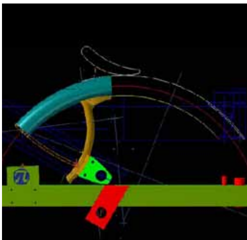
PiMoto aluminum monocoque in fixture drawing. Image courtesy of Pi Mobility.
