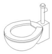
The 2D version of the toilet is invisible in a 3D view. Views of the toilet are available only in elevation and plan, which is sufficient for most project needs.
