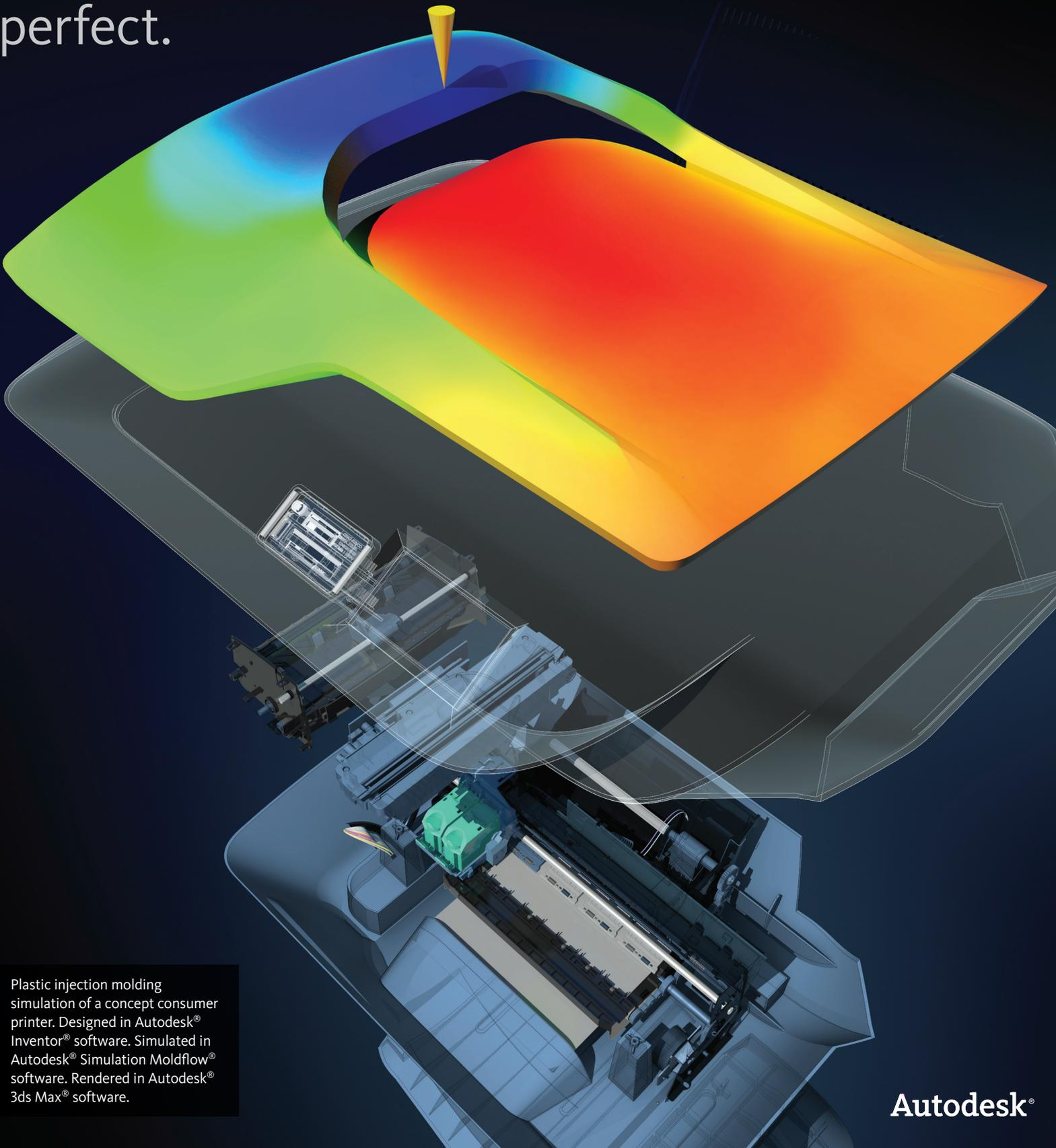
Plastic injection molding simulation of a concept consumer printer. Designed in Autodesk® Inventor® software. Simulated in Autodesk® Simulation Moldflow® software. Rendered in Autodesk® 3ds Max® software.
