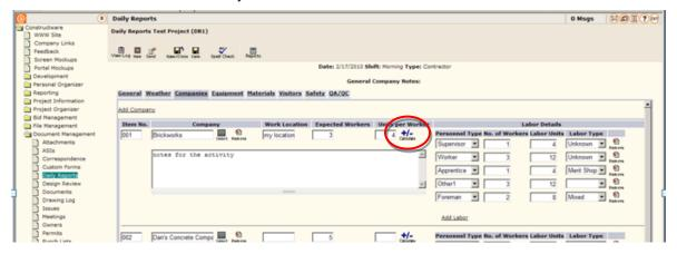
The number of labor units is calculated from the **No. of Workers** times the **Units per Worker**. If you change the amount entered in either field on the Companies window, click the **Calculate** button to recalculate this number. Clicking **Save** also invokes an automatic recalculation before the save.
