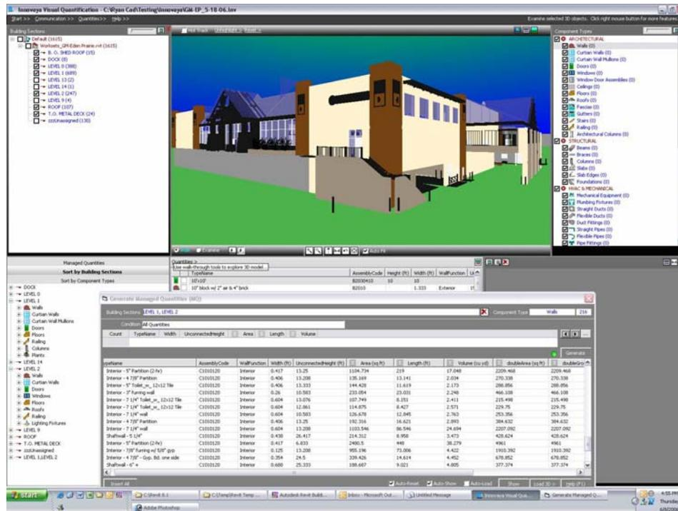
**Figure 2:** An API integration with Revit enables the Innovaya estimating solution to count and calculate materials directly from the Revit building information model.
