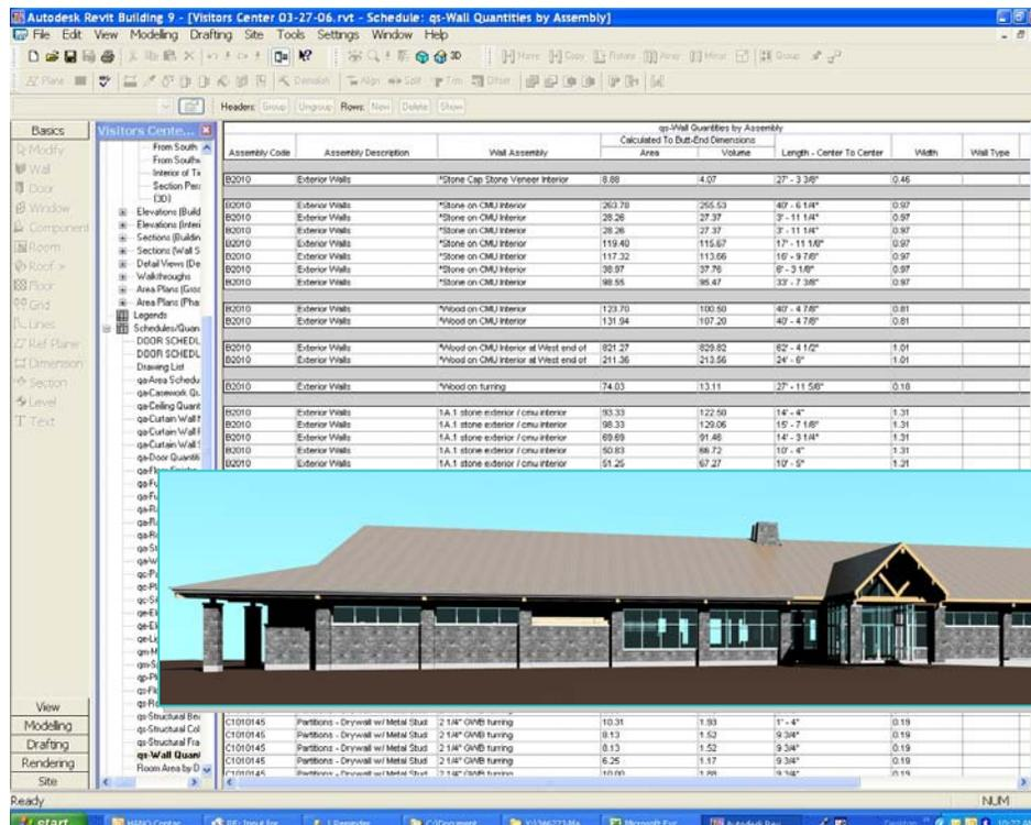
**Figure 5:** Parsons Brinckerhoff uses Revit to get accurate quantities much earlier in the design process.
