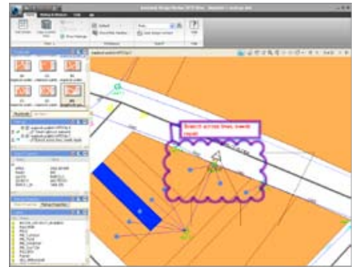
Markups made using Design Review are recorded in the Revit, Inventor, Civil 3D, or AutoCAD Markup Set Manager for easy navigation and quick revisions.
