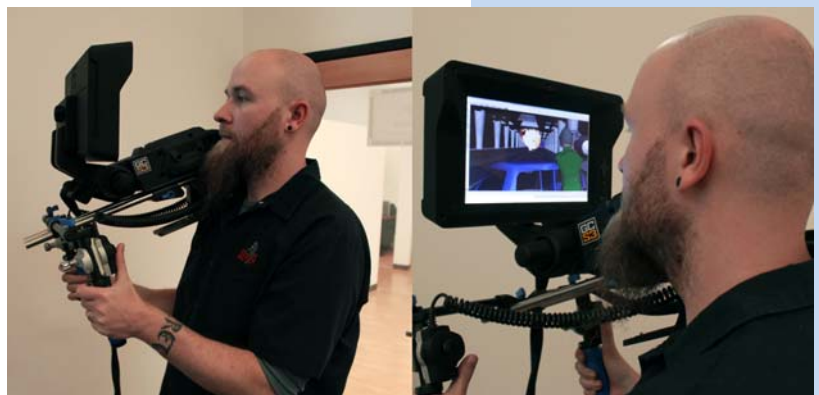
Fig 5c. Halon Previs Supervisor Justin Denton films a CG scene in Maya in real-time with the Gamecaster GCS3 virtual camera controller.
