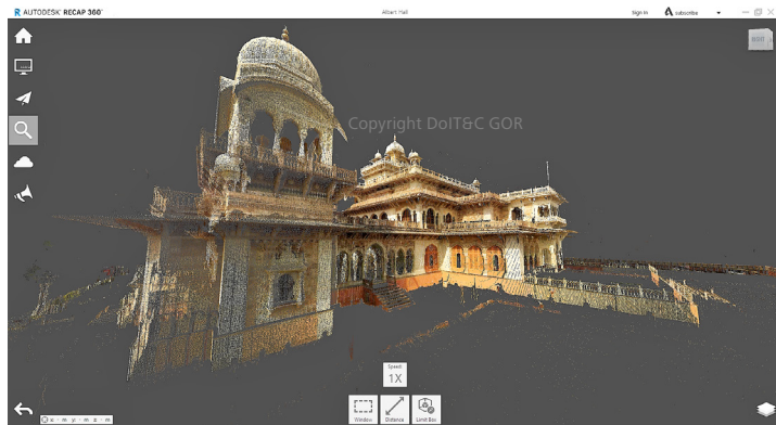
LiDAR point cloud data of Albert Hall in Autodesk ReCAP 360 Pro - Image Courtesy: DoIT&C
