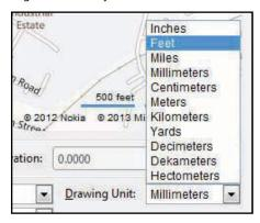
The selected coordinate system defines the scale of the map. You can easily modify the drawing units.
