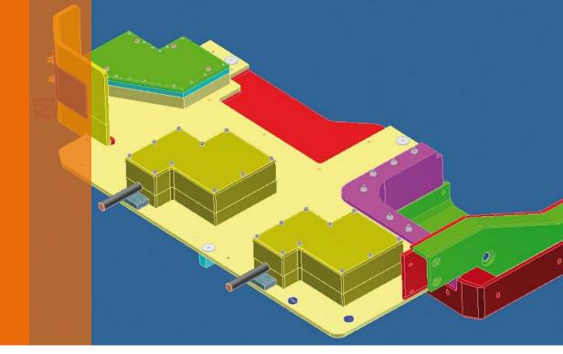
required panel shapes and then export these to our MasterCam software to generate CNC programs for the production machines."
