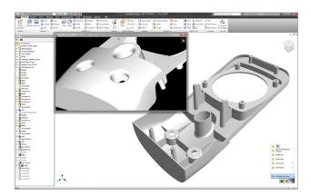
Beyond viewing the filling pattern, you can use the real-time results to view injection pressure, weld lines, and even sink marks. The Finished Part Preview displays these defects directly on the model; you can see how your finished plastic part will look, then make adjustments to the engineering features to make sure aesthetic requirements are met.
