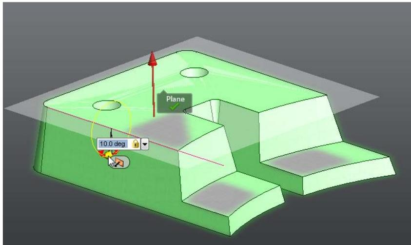
Finally, you OK the command to apply the draft to the model:
