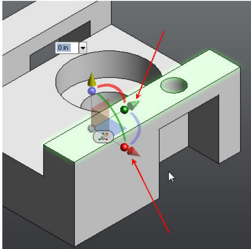
This planar face is not free to move in those directions. In some cases, the move command may not be able to detect these limitations, and manipulators are enabled, even though dragging in that direction does not result in a change to the model.
