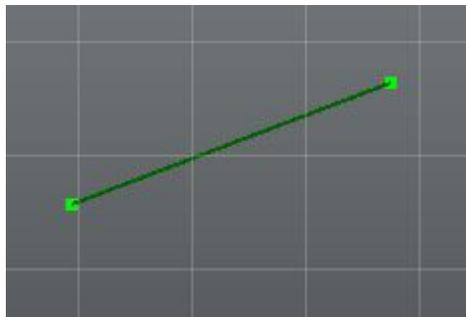
Locking a curve does not automatically lock its endpoints or vertices. When a curve is locked, it cannot be moved. In the previous image, the line is locked; however its endpoints are not. This reduces the edit operations you can perform on the curve and even on curves or points connected to it. In the previous example, you can extend the line in either direction, but you cannot move the position of the line or change its direction.
