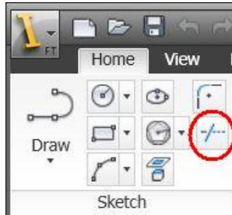
With this command, you can trim Sketch entities against other entities on the Sketch plane, or extend them to other entities. The command is in the Trim mode by default. You can switch to the Extend mode by using the drop-down menu (press the down arrow key). Invoking the drop-down menu again switches back to the Trim option.
