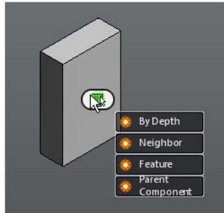
The Parent Component option directly selects the component which is the parent for the face edge. When you select By Depth, Neighbor, or Feature, a selection strip is displayed. The strip contains several frames each representing a possible selection.
