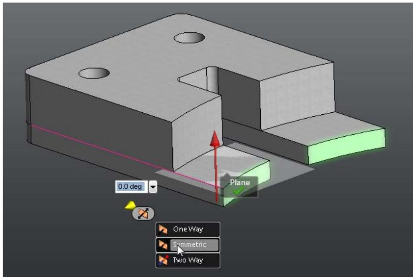
Drag or enter a draft angle. The result shows that the model has been split along the neutral plane, and the draft applied symmetrically to both sets of
