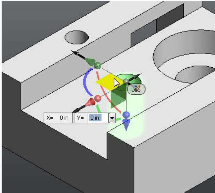
In this case, the highlighted plane manipulator can be used to move the selected cylindrical face in either the direction of the green arrow or the red
