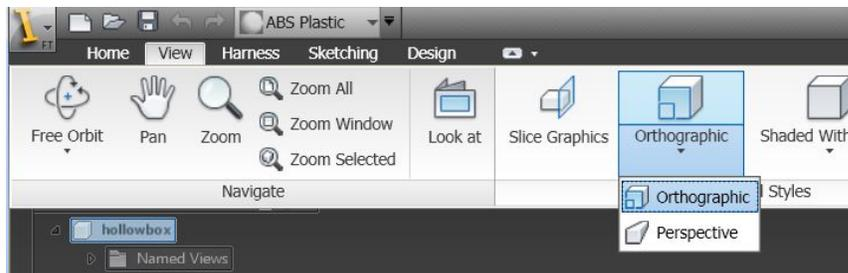
In Orthographic Camera mode, a model is displayed so all its points project along parallel lines to their positions on the screen. All same-length parallel edges display as the same length, even when you orient them so one edge is
