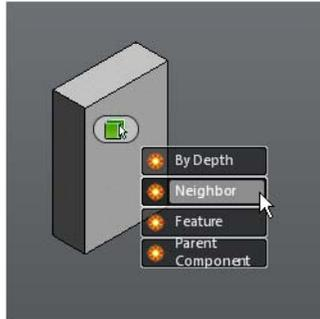
In the following example, the topological neighbors of a root face are listed in the selection strip. The last item in the strip represents all the edge loops connected with the root face.
