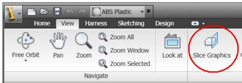
It can also be activated or deactivated by pressing the F7 function key. When Slice Graphics is active, it will cut any bodies that intersect the plane. It will also create temporary “caps” to close any holes created by the slicing action, as you can see in the following images.
