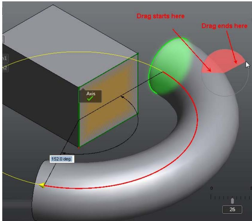
Next, change the Operation Type of the Revolve feature to create a new body. Click and hold down the left mouse button over the Operation Type glyph, and choose New Body.
