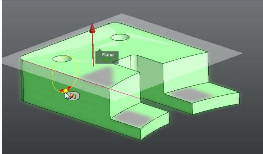
Next, you would drag, or enter a precise value into the draft angle entry box. In the following image, the draft angle has been set to an unusually high value, to more clearly show the effect of the draft operation.
