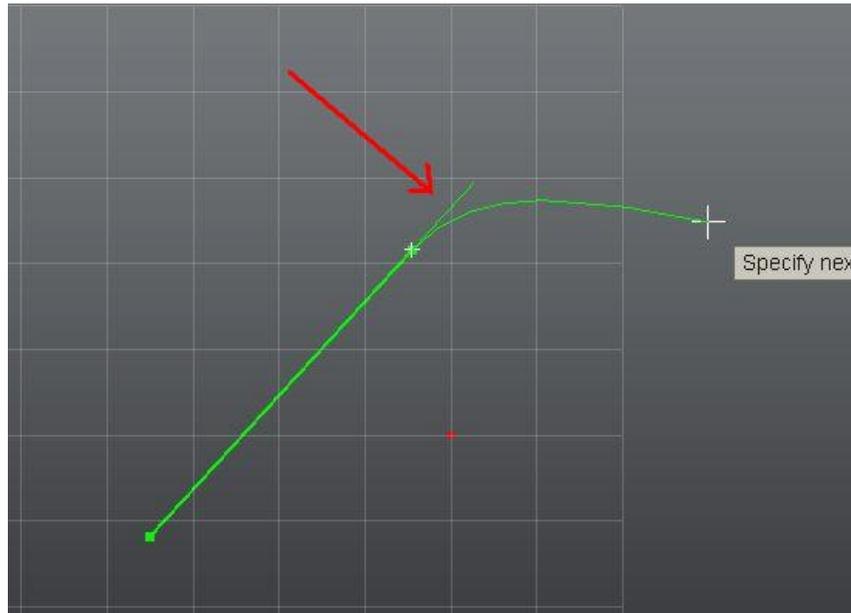
You can create open splines as well as closed splines. You can complete the creation of an open Spline entity by double-clicking at the last point. To create a closed Spline, click the start point of the current spline entity – it also is defined at the endpoint. The current entity creation is completed and you can start creating a new entity.
