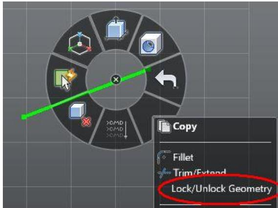
When an entity is locked, it is drawn in dark green. User-created edges are unlocked by default. [Projected Geometry](#) on page 157 is locked by default.
