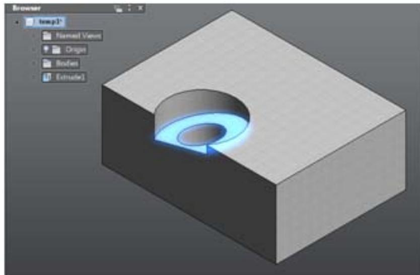
If a find features recognizes a feature in a way that does not fit your intent you can change it. In the browser you can right-click and change the feature type. For example recognize a hole as a revolve. You can also dissolve the feature which removes the feature from the browser but leaves the geometry on the model.
