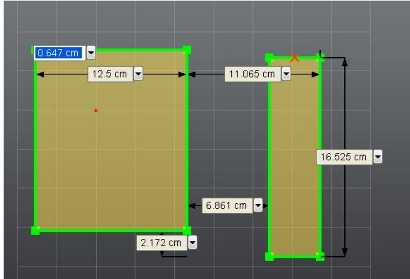
A red X appears on dimensions that are being edited. The X indicates which endpoint is fixed while the dimension is being edited. To lock or unlock a sketch entity, click the entity, then invoke the marking menu (RMB) and select Lock/Unlock Geometry from the context menu. See [Locking Sketch Geometry](#) on page 176 for more information.
