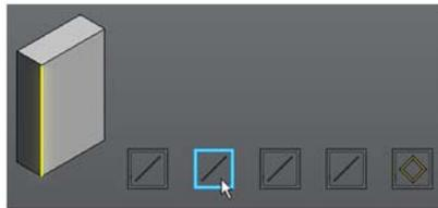
When you highlight a frame in the selection strip, the corresponding edge element is also highlighted.
