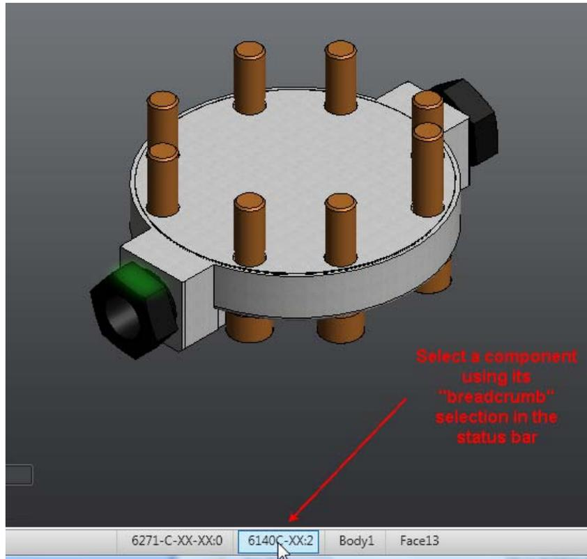
Once the component is selected, use the Move command's manipulators to translate or rotate a component. Note that if other components have constraints to the component being moved, they will also move to satisfy the constraints.
