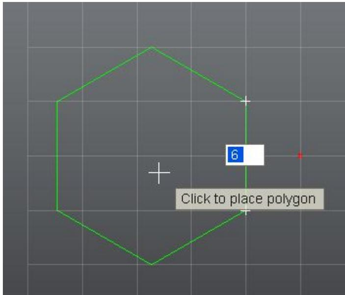
You can also switch between the different Polygon creation options from the drop-down menu that is available when you are not in the middle of a creation operation. Press the down arrow key to get this option.
