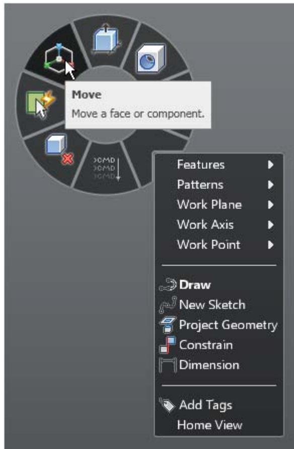
The marking menu item for Move is highlighted and the commandtip for the highlighted item is shown.
