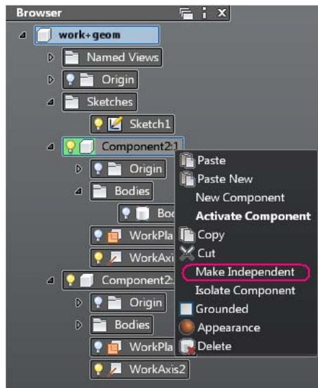
This command makes the subassembly represented by the component instance “independent”, for example, it is equivalent to a cut followed by a deep copy of the component instance in the same parent container.
