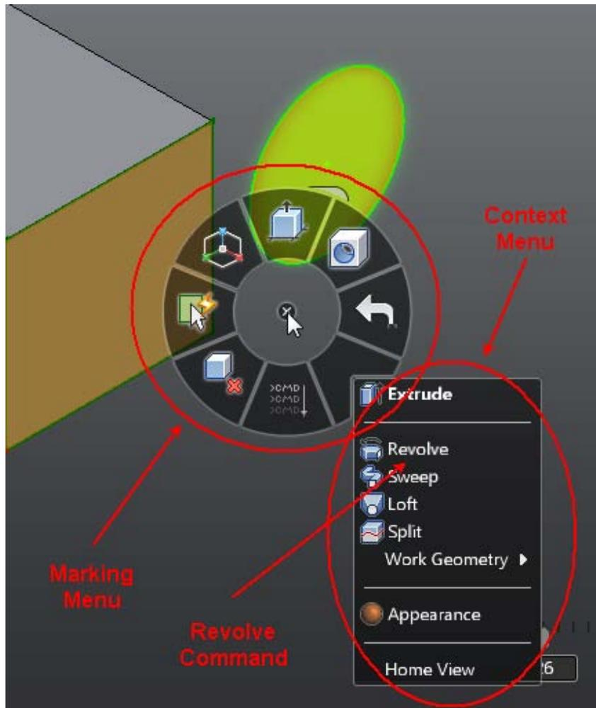
This brings up the Revolve command, with the circular region as the profile to Revolve.
