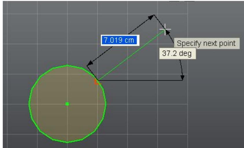
This is very similar to the Tangent Constraint, except that it is inferred when you move/drag in a direction perpendicular to the circle or circular arc.
