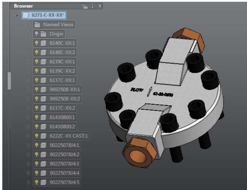
Components in Inventor Fusion are organized hierarchically. That is, each component can have zero or more child components, and those child components can have child components, and so on.
