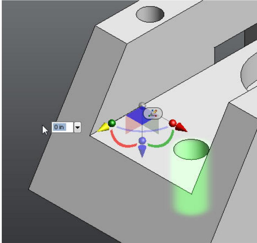
Translate manipulators can be reoriented along linear edges, work axes, cylinders, and planar faces. The triad can be reoriented about an active rotate manipulator similarly. Reorienting about a rotate manipulator is identical to reorienting about the corresponding translate manipulator. For instance, the blue rotate manipulator corresponds to the blue translate manipulator.
