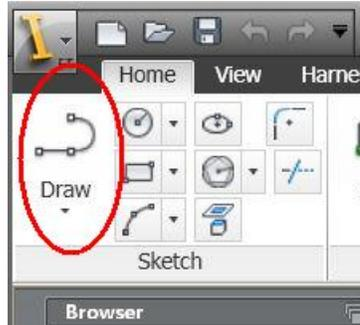
When you activate the Line/Arc command, you can define points by clicking the mouse, or by typing the values into the Heads-Up Display (HUD) text boxes. When relevant, you get HUD text boxes where you input line lengths and angles from the vertical/horizontal. This helps you to create more precise geometry. You can press the TAB key to navigate from one HUD text box to another.
