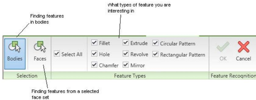
In the following image, Find Features adds an extrude (the rectangular body) and a counter bore hole (the cylindrical cut) to the browser. Once a feature has been found, it is managed the same as features created with traditional methods. Features can be edited, deleted or dissolved.
