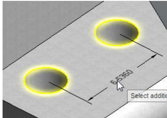
Two circular edges, concentric and not coplanar
