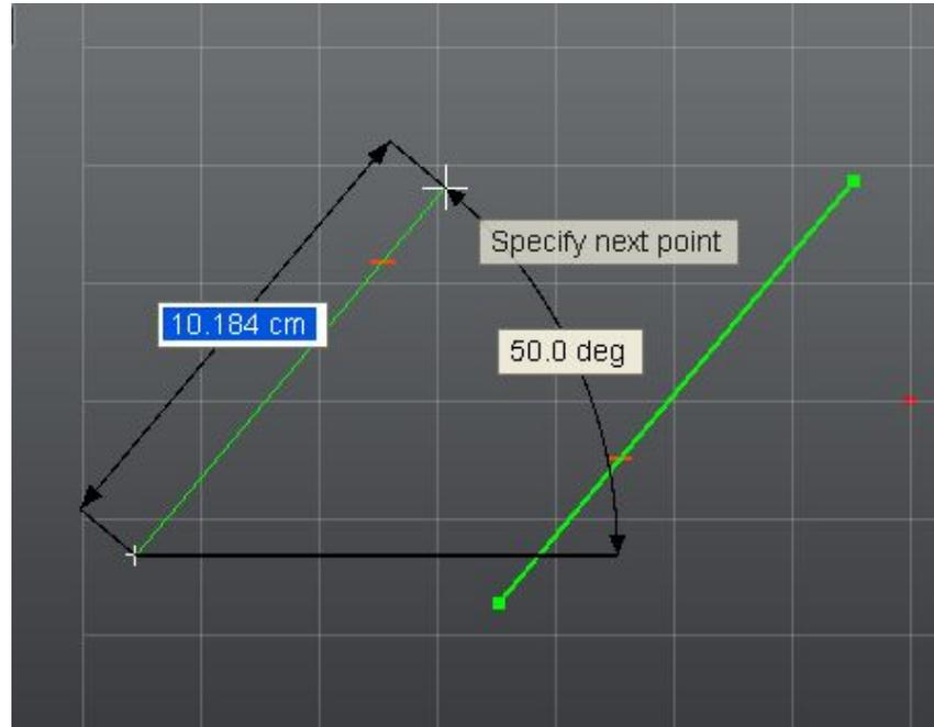
A parallel constraint is inferred when you “touch” a line that does not share endpoints with the line you are currently trying to create, and then moving your mouse in a direction roughly parallel to that line. Your line will be adjusted to be parallel to the “touched” (referenced) line and you will see a red horizontal line symbol on both the line being created and the “touched” line.
