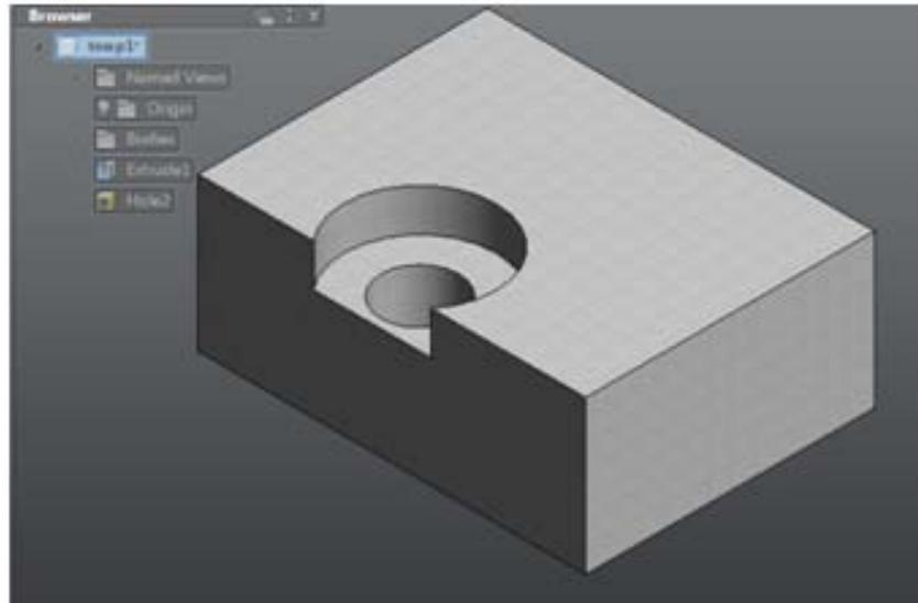
If a downstream operation modifies a feature face, the owning feature will be re-evaluated. If the face set does not satisfy the feature definition, the feature will be removed from the browser. In the previous counter bore hole example, if the user moves the highlighted face, the feature will not be a valid counter bore hole and is removed from the browser at the end of move operation.
