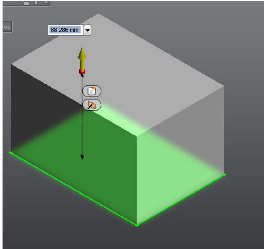
Finish the command. There are a couple of ways to complete the command - starting another command, or clicking OK in the ribbon. In this case, click OK in the ribbon. This creates the body, as well as an Extrude feature in the browser:
