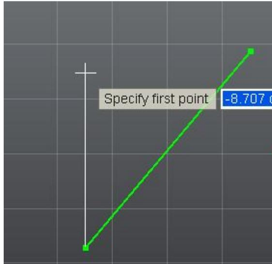
Another kind of vertical constraint can be inferred by “touching” a point and moving the mouse in a vertical direction. You will see a white line stretching from the “touched” (referenced) point to your current mouse position. This means that the point that your command is in the process of defining is constrained to have the same Y-axis value as your “touched” point.
