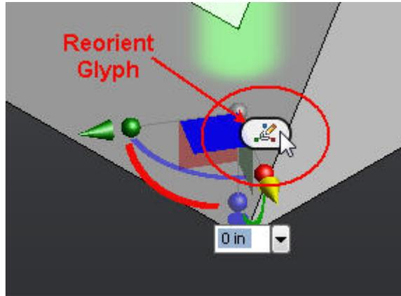
If you click this glyph, the move command enters reorient mode. In this mode, geometry selections are used to reorient the triad, by aligning the active triad manipulator with the selected geometry. If a translate manipulator is active, a linear edge can be selected, and the triad is moved so that the active translate manipulator is aligned with the edge. For instance, if the
