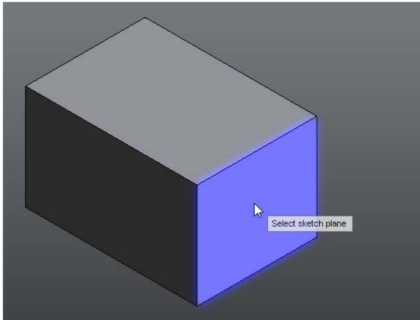
This creates and activates a new sketch, changes the view to look at the new sketch, and invokes the Circle command. Select a circle center and radius point, away from the existing body. Note that because we selected a face of the existing body, Fusion has generated sketch geometry that coincides with the edges of that face. This sketch geometry is fixed, and so can't be edited.
