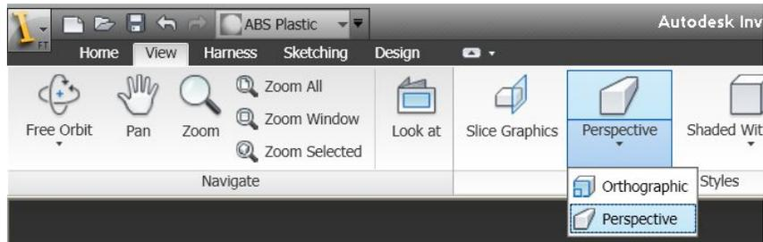
In perspective camera mode, the model is displayed as it would be seen with a human eye. Objects further away from the camera appear smaller than objects closer to the camera. Also, if two lines are parallel to each other and are along the line of sight, they will appear to converge as they move further away from the camera.
