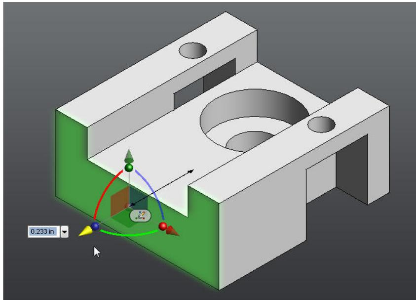
Move can be applied to geometry of any kind. In this example, one of the cylindrical holes is translated along one side of the model:
