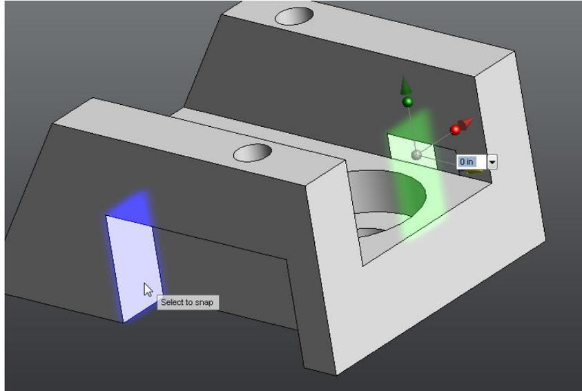
Use the Move command to achieve this with its snap to geometry feature. When a face is selected, if an applicable face is clicked that can be snapped to, move transforms the active faces so that they are aligned. Inventor Fusion indicates that snapping is possible with the prompt Select to snap when the cursor is over an available snap face. In the previous case, the selected green
