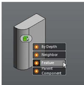
In the following example, both the extrusion and the fillet are eligible features. The icons on the selection strip make it easy to identify the features by type.
