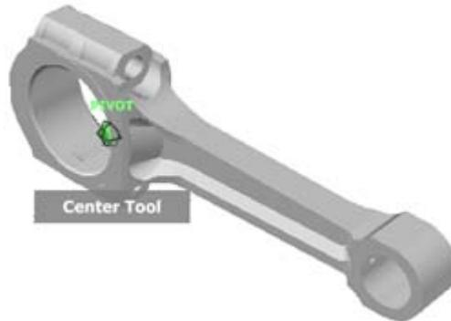
The point defined by the Center command provides a focal point for the Zoom command and a pivot point for the Orbit command.
