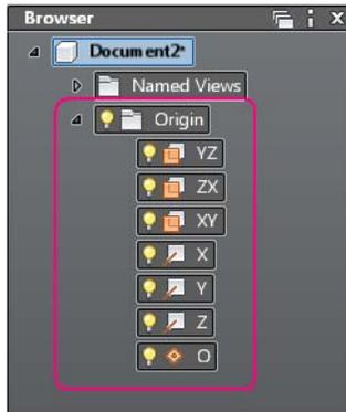
The three default work planes are the YZ, ZX, and XY planes. The three default work axes are the X, Y, and Z axes. The single default work point is the O point which represents the value 0, 0, 0 in the model. The default work planes and axes are based on the origin point. The following image shows the origin geometries in the graphics window.
