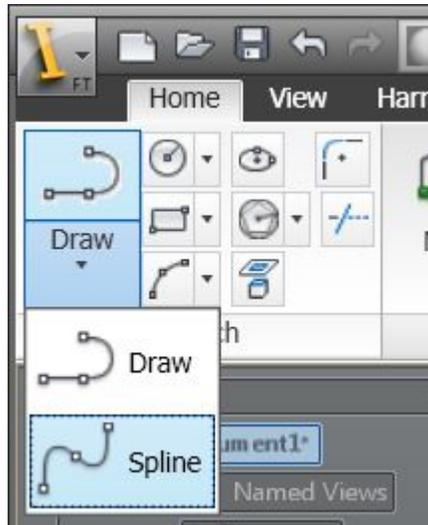
When you activate the Spline command, you can define fit points by clicking the mouse, or by typing the values into the Heads-Up Display (HUD) text boxes. This helps you to create more precise geometry. You can press the Tab key to navigate from one HUD text box to another.
