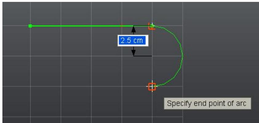
To create a line perpendicular or tangent to a circle or arc, click and hold the start point. Then drag the cursor to end the line segment. Drag the cursor
