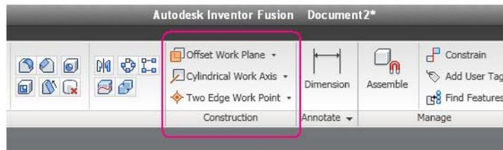
Create work geometry by selecting a work geometry command then selecting existing geometry. Except for Offset Work Plane and Angle Work Plane, no values are required to create work geometry. The geometry you select defines the position of the work geometry.
