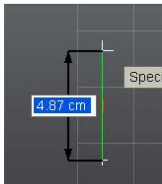
A vertical constraint is inferred if you are drawing a line and drag your mouse such that the line is parallel to the Y-axis of the Sketch Plane. It is indicated by a vertical red line symbol.
