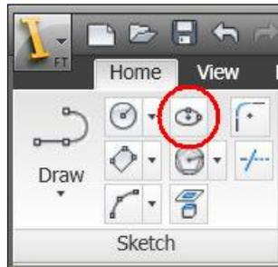
You can define an ellipse by picking the center point, followed by another point to define the major axis and finally a third point to place the minor axis.
