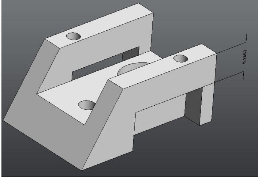
If the top face of the design is selected in the Move command, the dimension is honored, and so the bottom face moves along with the top face:
