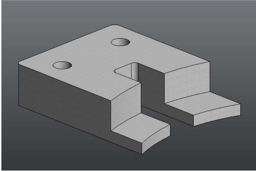
Invoke the Draft command. The first input this command requests is a neutral plane. This selection serves two purposes: It specifies the plane around which faces are drafted, and it also specifies the pull direction. That is, the direction in which the mold is removed from the part, after the molding process is complete. The second input is the faces to be drafted.
