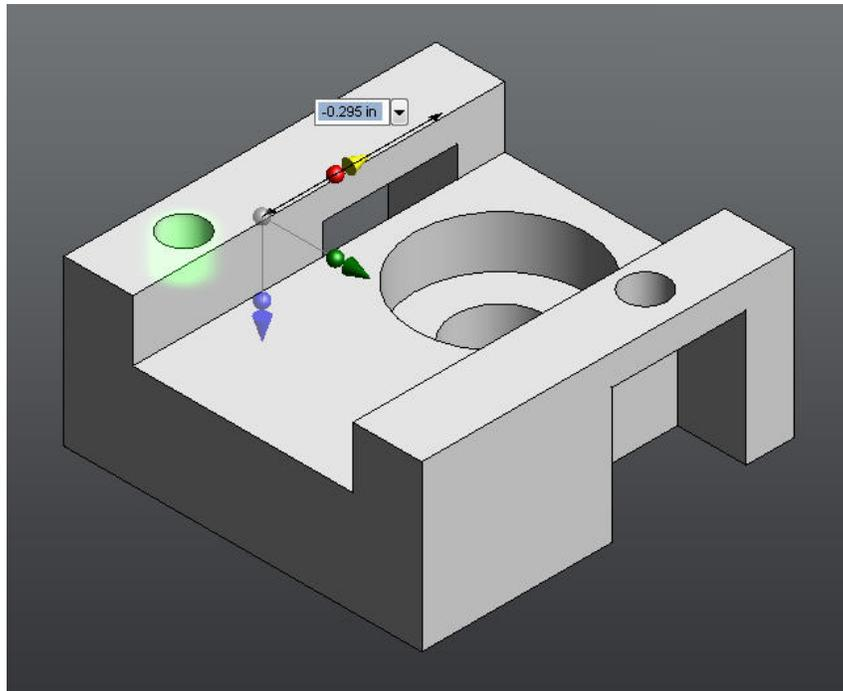
**Note:** Some faces are limited in their ability to move, by the geometry of the model. Note that in this case the red and green translation manipulators are
