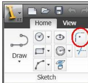
With this command, you can create fillets between two intersecting lines, two parallel lines, a line and a circular arc that intersect, and two circular arcs that intersect. Fillets can't be applied to circles, ellipses, elliptical arcs and splines. Fillets also can't be applied to non-intersecting entities, with parallel lines being an exception.
