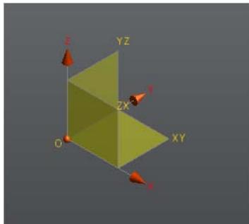
**Note:** The origin geometries are not visible by default. When a new [sketch](#) on page 135 is started, the geometries are displayed automatically. Use the light bulb icon to manually control the visibility of planes, axes, and point.
