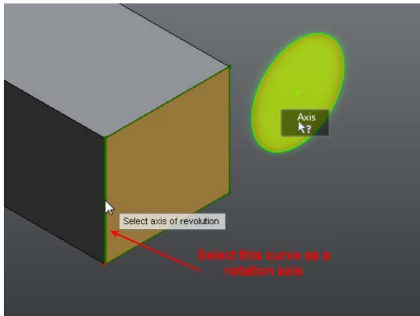
Once the axis is selected, begin dragging. In this example, we will drag in an area that is away from the manipulator. Click and drag the left mouse button in an area of the screen that is not over any graphics. The example drags to
