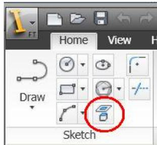
With this command, you can project model edges, work geometry and even Sketch geometry from other Sketch Planes onto your current Sketch Plane. Projected geometry is locked by default. See [Locking Sketch Geometry](#) on page 176 for further information on this topic.
