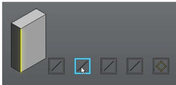
When you hover over a frame in the selection strip, the corresponding element is highlighted in the model. When you click a frame in the selection strip, the corresponding element is selected.
