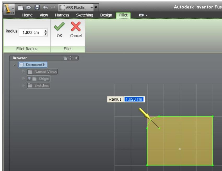
You can click and drag on the yellow arrow to define the fillet radius. You can also type into the Radius edit box to change the fillet radius.
