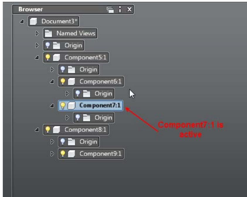
There are two ways to activate a component: Double-click the component's browser node, and using the Activate Component command.
