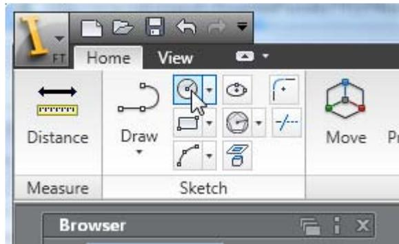
Because no sketch is currently active, the first step is to create a new sketch. Select a face of the existing body.
