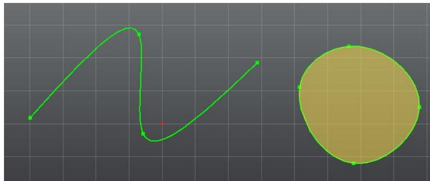
**Note:** It is possible to create self-intersecting splines (like a figure-8) using the spline command, but such non-manifold entities are not supported by the [Sketch Profile](#) on page 171 recognition system, and may cause undesirable results.
