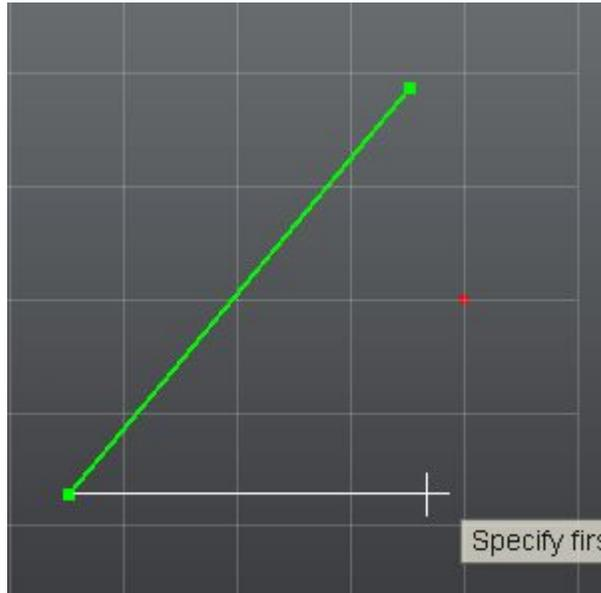
Another kind of horizontal constraint can be inferred by “touching” a point and moving the mouse in a horizontal direction. You will see a white line stretching from the “touched” (referenced) point to your current mouse position. This means that the point that your command is in the process of defining is constrained to have the same X-axis value as your “touched” point.
