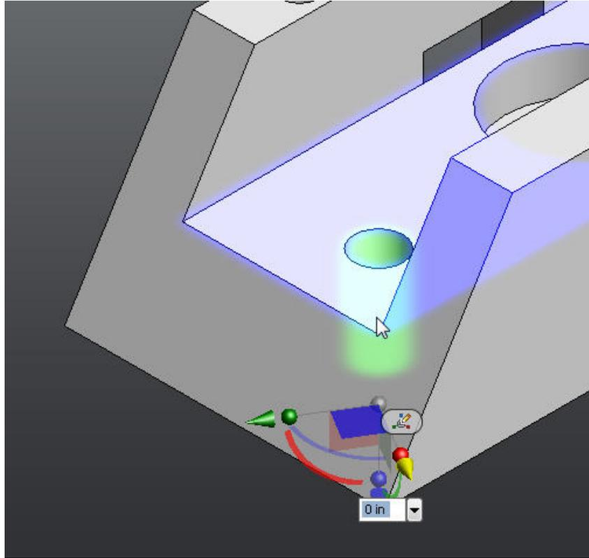
However, the default orientation is not ideal for moving the face along the rectilinear face that the hole is on. So, to change the default orientation to more fit your intended design modification.
