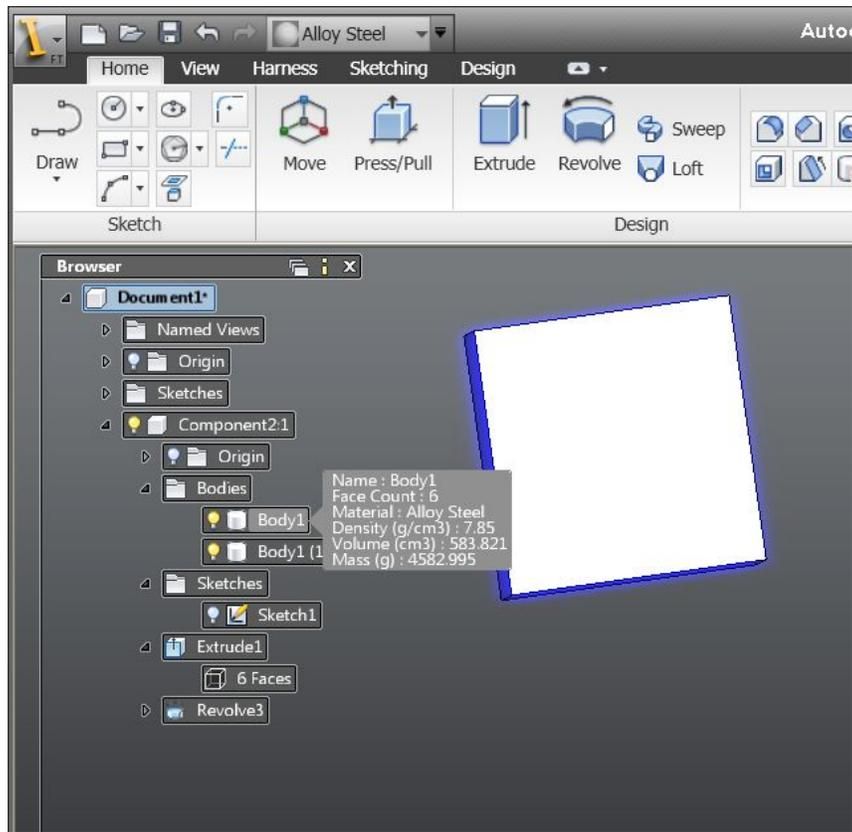
A body or component typically inherits the Material of its immediate parent. You can set the entire document to have a particular material, and any object created under it will have that Material. You can override the material of child objects by selecting them and using the drop-down menu available in the Quick Access commandbar.
