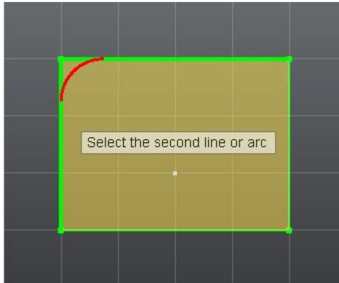
Highlighting another valid entity removes the existing preview and show you a new preview. If two entities can be filleted in more than one way (e.g. two lines intersecting to form an X have four possible fillet options) then the selection pick points determines which solution is created. See [FilletPreview.avi](#) on page 160 for a demonstration.
