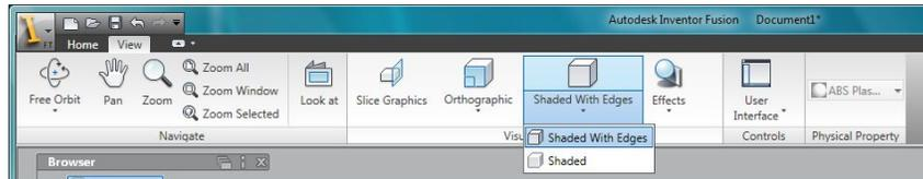
The Shaded With Edges option will draw both faces and edges. The Shaded option will only draw faces. Inventor Fusion does not support a Wireframe (Edges-only) style at present.
