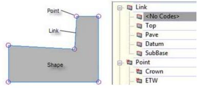
The fundamental components of subassemblies are points, links, and shapes. (Figure 3). Points are connected
