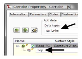
Figure 8. Codes can also be used when creating or extracting data from the corridor model. This example shows a finished grade surface reading the Top codes to create contours from the model.
