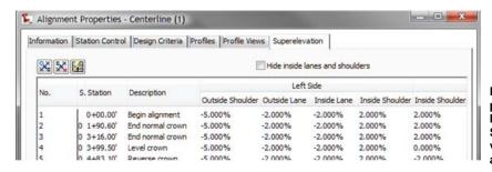
Figure 16. Superelevation parameters can be applied during the layout of the horizontal alignment. Subassemblies can then use these values as the superelevation is being applied throughout the design.
