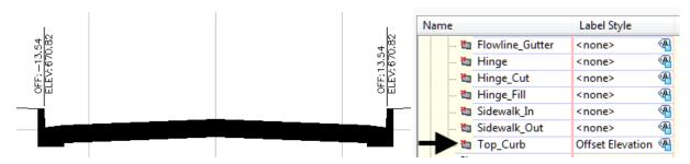
Figure 9. This example shows Top\_Curb codes being used to label cross sections. Offsets and elevations are automatically derived from the corridor model and conform to company or jurisdictional CAD standards.
