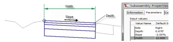
Figure 4. Input parameters allow specific components within subassemblies to be customized to fit specific project requirements. The example shown will create a lane 12' wide with a cross slope of 2% and a material course depth of 0.67 feet for the duration of the road.
