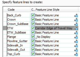
Figure 7. Each feature line can be assigned a style to control the display, for that part of the corridor.
