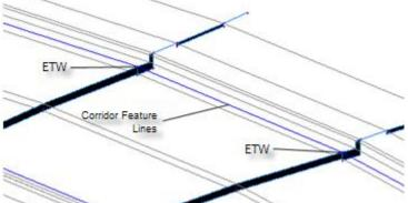
Figure 6. Corridor feature lines will automatically connect ETW points as the corridor is created.
