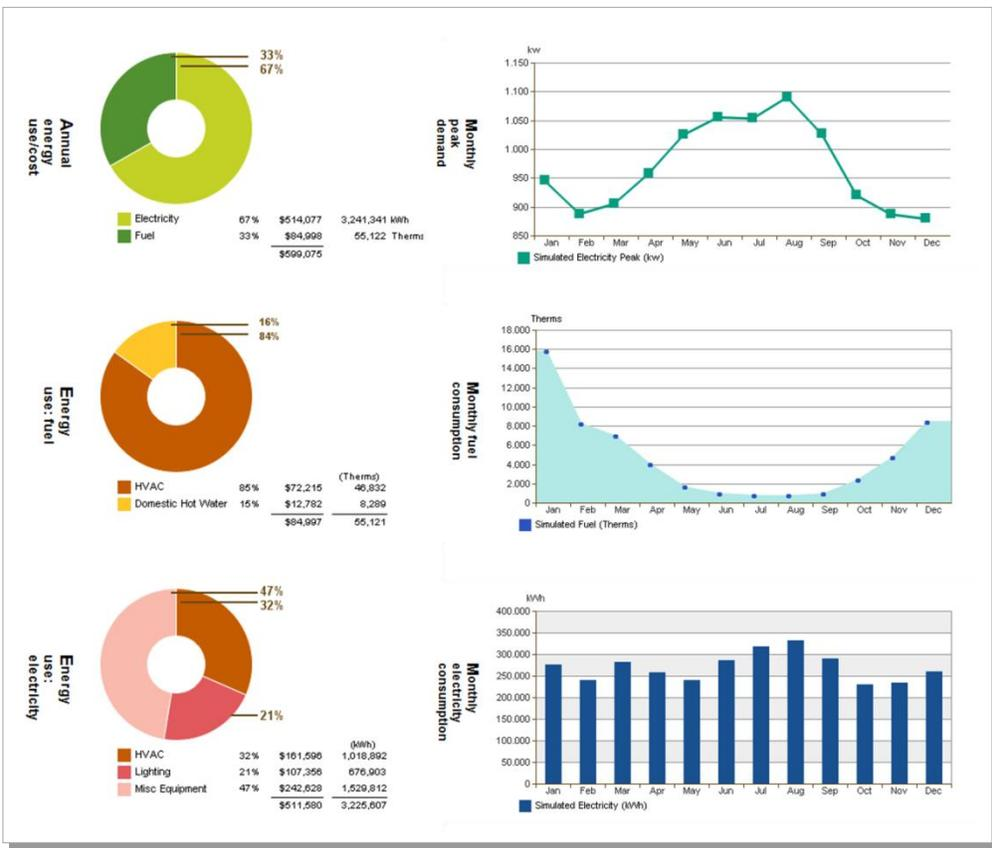
Figure 5: Autodesk Revit Conceptual Energy Analysis features help you simulate your building performance.
