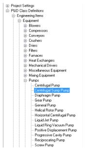
Continue to expand the list until you locate and select *Engineering Items* ➤ *Equipment* ➤ *Pumps* ➤ *Centrifugal Sump Pump.*
