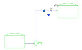
**2** Drag the gate valve from the horizontal line, and click on the vertical line to place the valve.
