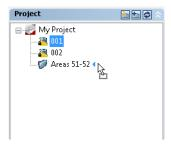
4 Click and drag drawing 002, and place it into the Areas 51-52 folder, under drawing 001. If necessary, drag drawing 001 above drawing 002.
