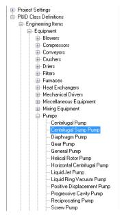
**3** Continue to expand the list until you locate and select *Engineering Items* ➤ *Equipment* ➤ *Pumps* ➤ *Centrifugal Sump Pump.*
