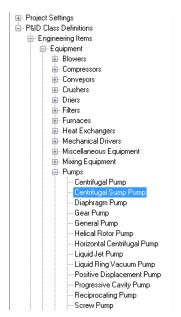
**5** Continue to expand the list until you locate and select *Engineering Items* ➤ *Equipment* ➤ *Pumps* ➤ *Centrifugal Sump Pump.*
