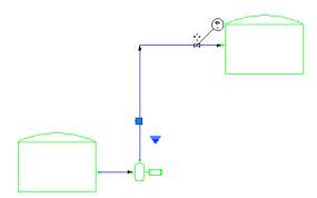
**3** Right-click the gate valve and click Deselect All to see that the valve has flipped to align with the vertical line.
