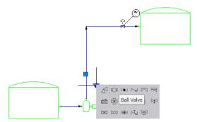
3 Click Ball Valve (the second valve in the list). The gate valve is replaced by the ball valve.
