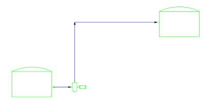
**Note** To view a flow-direction error, start the schematic line at the pump and end it at the tank. You can then reverse the flow to fix the error. To reverse the flow, right-click the line and select Schematic Line Edit ➤ Reverse Flow.
